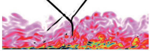
Figure 4: Instantaneous close-up view of the mixing layer with consecutive vortex shedding in the separated region. Vorticity magnitude contours (colored) and shock structures (black) at side-plane.
