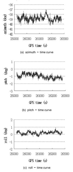
Fig. 3 Results of AMES for conplanar configuration
