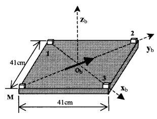
Fig. 2 TANS Vector's 4-antenna square configuration
