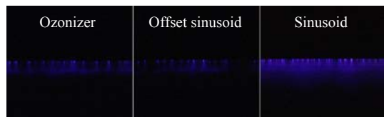
Fig. 17 Over-head photos of discharge region ( V=6\text{kV}_{\text{p}} ).
