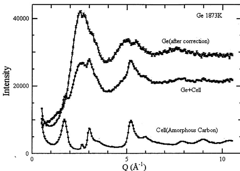
Fig. 3. The neutron scattering experiment of liquid germanium at 1873 K with the use of an amorphous carbon container.
