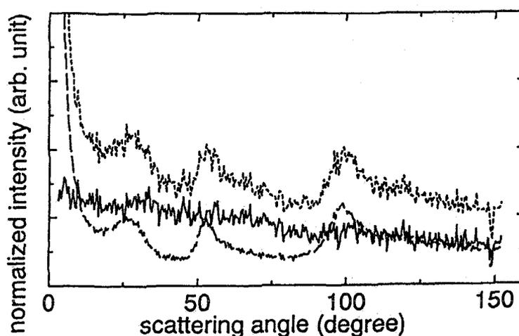
Fig. 2. Temperature dependence of the neutron total scattering spectrum of the amorphous carbon cell. The dotted line correspond to the spectrum at room temperature and the broken line is at 1273 K. The solid line corresponds to the difference between them.
