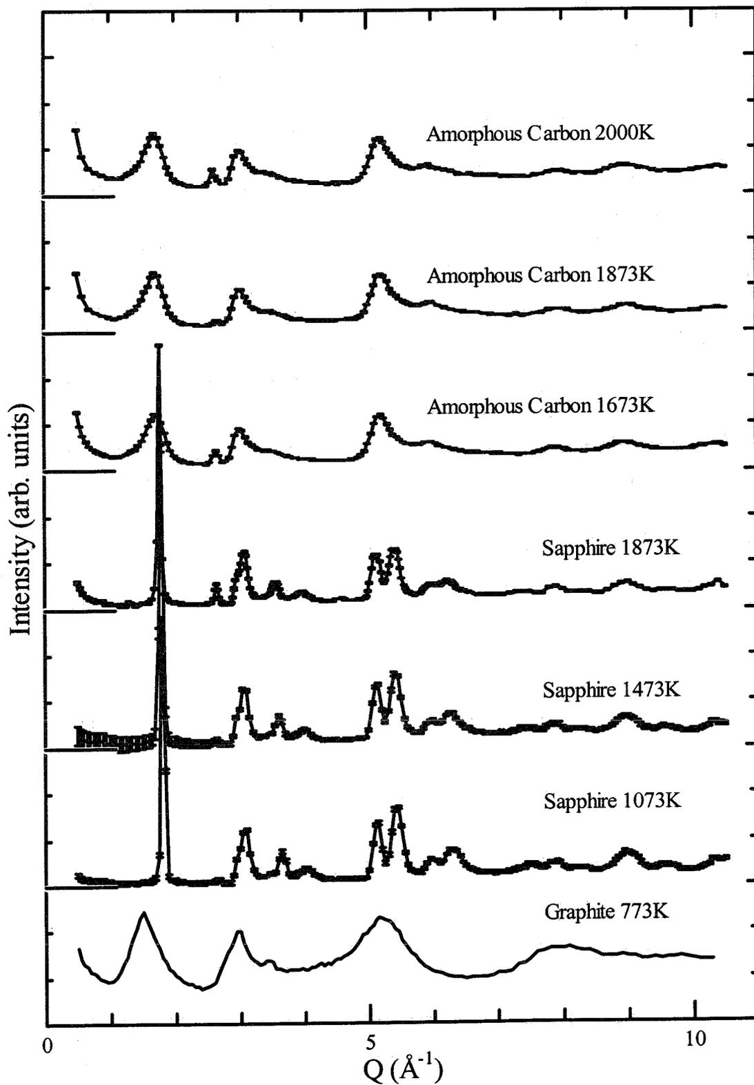
Fig. 1. Neutron total scattering spectra of the containers. The measurements have been done by TAS-1 spectrometer at JAERI, Japan.
