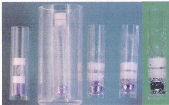
Figure 2 Ampoule after seal material test: (a) Before experiment, (b) 360 Torr, (c) 560 Torr, (d) 760 Torr, (e) 1140 Torr.
