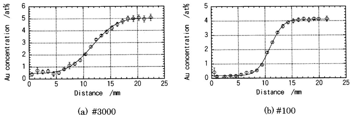
Fig.2 Concentration distribution after diffusion experiments with #3000 and #100 finished shear cell disks respectively
