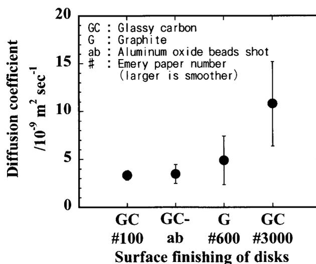
Fig.3 Effect of surface roughness of shear cell disks
