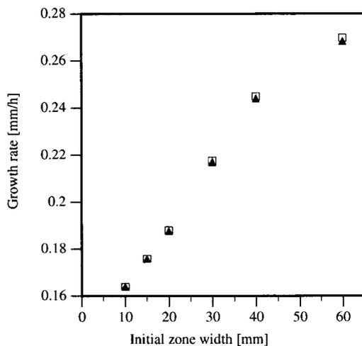
FIG.6 Steady-state crystal growth rate at the center of the seed crystal–solution interface. The depth of the solution is 10 mm and the initial temperature gradient in the solution is 10 K/cm.
