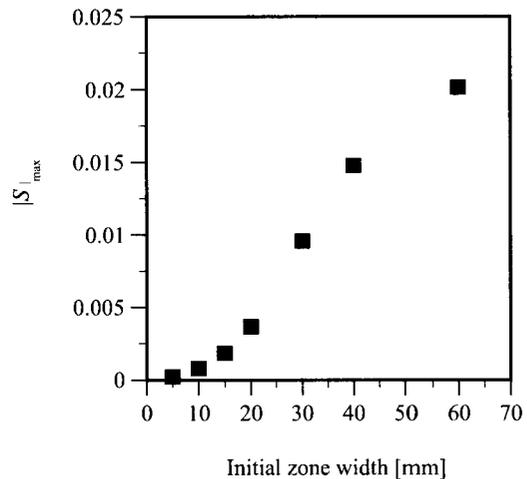
FIG.10 Dependence of the degree of supercooling on the initial solution zone width. The depth of the solution is 10 mm. The initial temperature gradient in the solution is 10 K/cm.  $1\ \mu\text{g}$  is applied.
