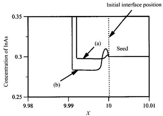
FIG.9 Distributions of the solute concentration along the center of the grown crystal. The depth and the zone width of the solution are 10 mm.  $1\ \mu\text{g}$  is applied.  $\tau = 3$ . (a) The initial temperature gradient in the solution is 10 K/cm; (b) 20 K/cm.
