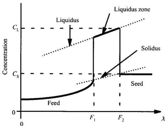
FIG.1 Traveling Liquidus Zone method. A linear concentration distribution is established in the solution and crystal grows naturally following Eq.(1). Therefore, if the heater is moved at the spontaneous crystal growth rate, a crystal of uniform compositions can be grown.
