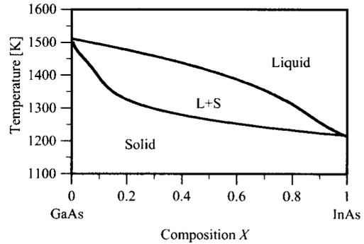
FIG.2 Pseudo-binary phase diagram of InAs–GaAs.
