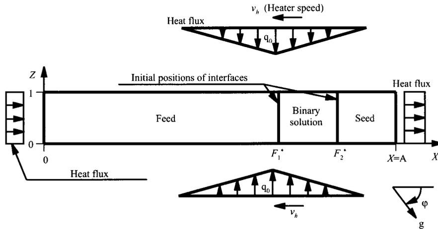
FIG.3 Outline of a crystal growth model of a binary InAs–GaAs semiconductor. A solution is sandwiched between seed and feed crystals. Heat flux is given externally from the top and bottom surfaces and the left-hand side wall. Heat is removed from the right-hand side wall. The velocity, temperature and concentration fields and the shape and movement of the interfaces are calculated numerically.
