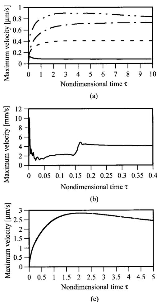
FIG.4 Time variations of maximum velocity in the solution. The temperature gradient in the solution is 10 K/cm. (a) The depth of the solution is 10 mm. The residual gravity is 1  $\mu$ g. — : the solution zone width is 10 mm; - - - - - : 20 mm; - · - · - : 40 mm; · · · · · : 60 mm. (b) The depth of the solution is 10 mm. A terrestrial gravitational acceleration of 1 g is applied. (c) The depth of the solution is 20 mm and the solution zone width is 40 mm. The residual gravity is 1  $\mu$ g.
