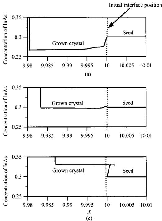
FIG.8 Distributions of the solute concentration along the center of the grown crystal. The depth of the solution is 10 mm and the initial temperature gradient in the solution is 10 K/cm.  $1\ \mu\text{g}$  is applied. (a) The initial zone width is 20 mm;  $\tau = 3$ ; (b) 10 mm;  $\tau = 7$ ; (c) 5 mm;  $\tau = 7$ .
