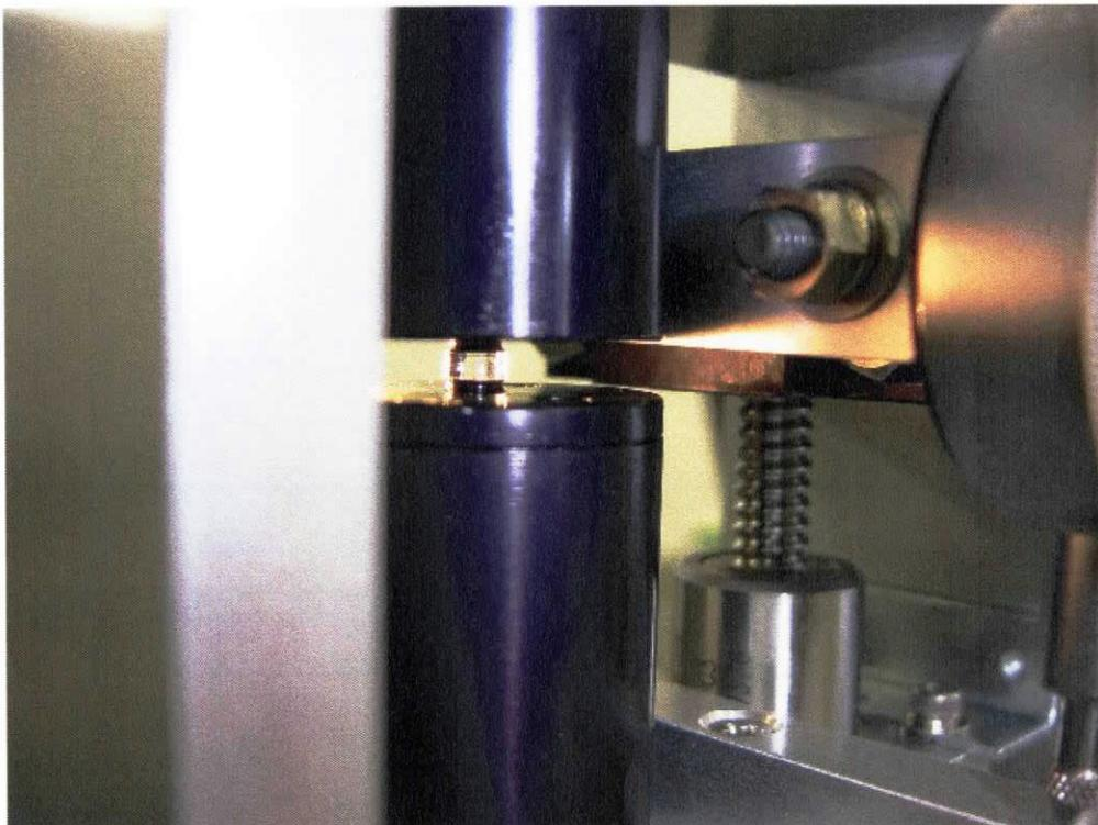
Figure 2.3-6 Small liquid bridge formation test
