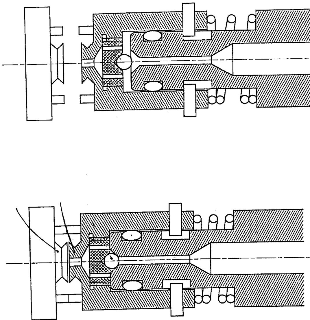
Figure 2.1-2 Inner ball seal type
