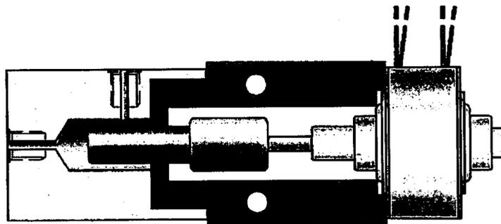
Figure 2.3-1(b) Cut image of variable volume pump
