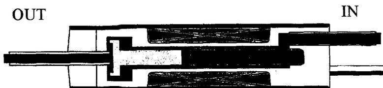
Figure 2.3-2(b) Cut image of micro valve
