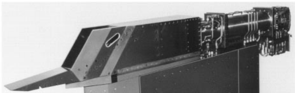
Fig. 4.7.1 The \text{CH}_4 -fueled ramjet engine tested in RJTF for the HYPR combined engine project.
