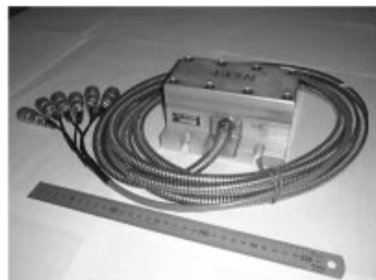
Fig. 7.2.1 The 6-component load cell used in the subscale wind tunnel.
