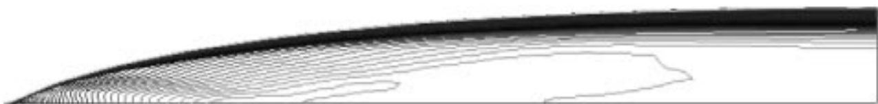
図1.7 Numerical calculation result for Mach contour in Mach 6.7 nozzle.
