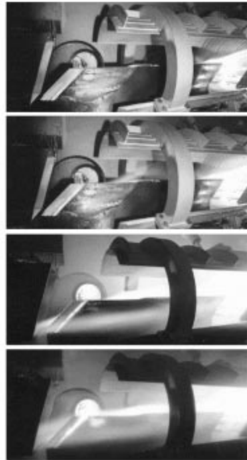
Fig.6.11 Diffuser breakdown observed in a Mach 8 engine test in the RJTF
