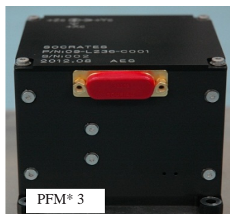
Fig. 4 VSGA (Vibrating Structure Gyroscope Assembly)
