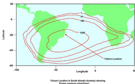
Fig. 14, ERS-1/PRARE Failure location, proton latch-up.
