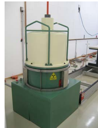
Fig. 7. ESTEC Co-60 gamma source inside the shielding chamber (photo courtesy by Bob Nickson).
