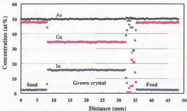
Fig. 1. Compositional profiles of a TLZ grown crystal at a sample translation rate of 0.22 mm/h. Crystal diameter is 2 mm.
