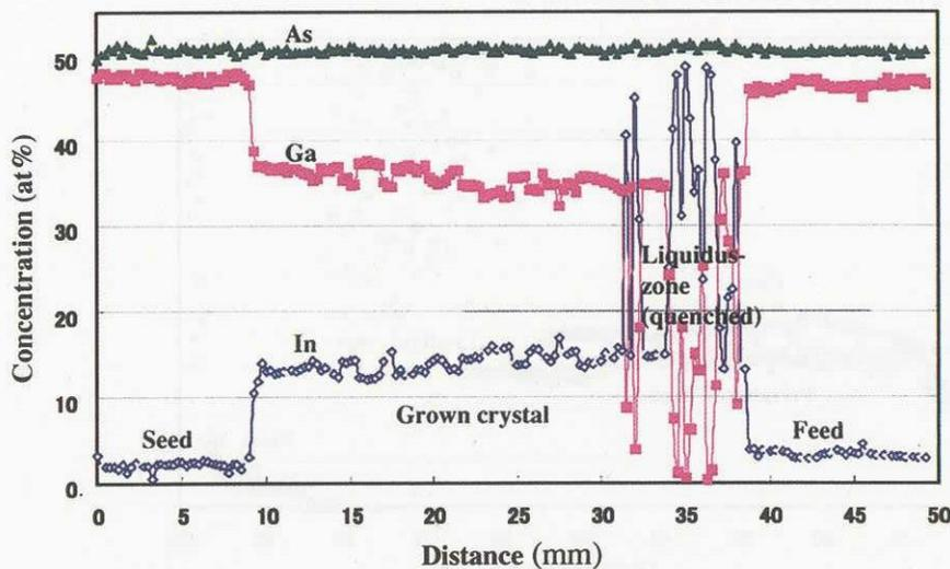
Fig. 4. Compositional profiles of a TLZ grown crystal at a sample translation rate of 0.32 mm/h (45% higher than the critical growth rate).
