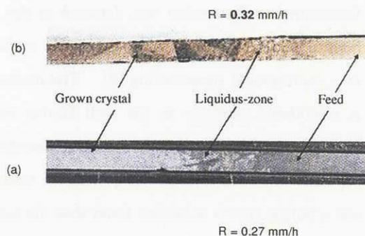
Fig. 5. Cross sectional view of TLZ grown crystals; (a) sample translation rate  $R = 0.27$  mm/h and (b)  $R = 0.32$  mm/h. Polycrystallization occurred at  $R = 0.32$  mm/h.
