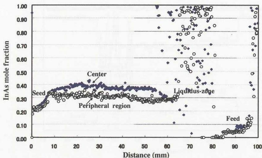
Fig. 6. Compositional profiles of a TLZ grown 10 mm diameter crystal at a sample translation rate of 0.22 mm/h.
