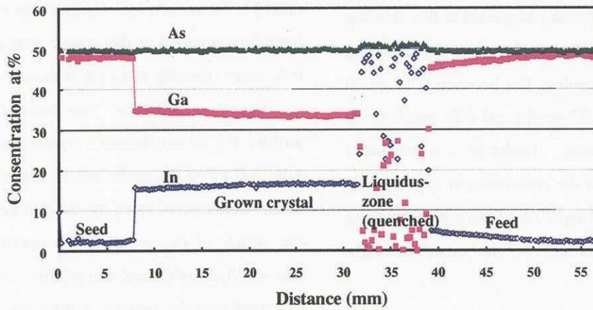
Fig. 3. Compositional profiles of a TLZ grown crystal at a sample translation rate of 0.27 mm/h (23% higher than the critical growth rate).
