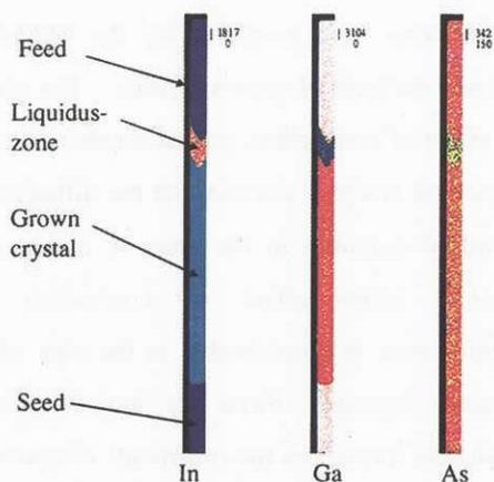
Fig. 2. EPMA mapping of In, Ga and As distributions for a TLZ grown crystal at a sample translation rate of 0.22 mm/h.
