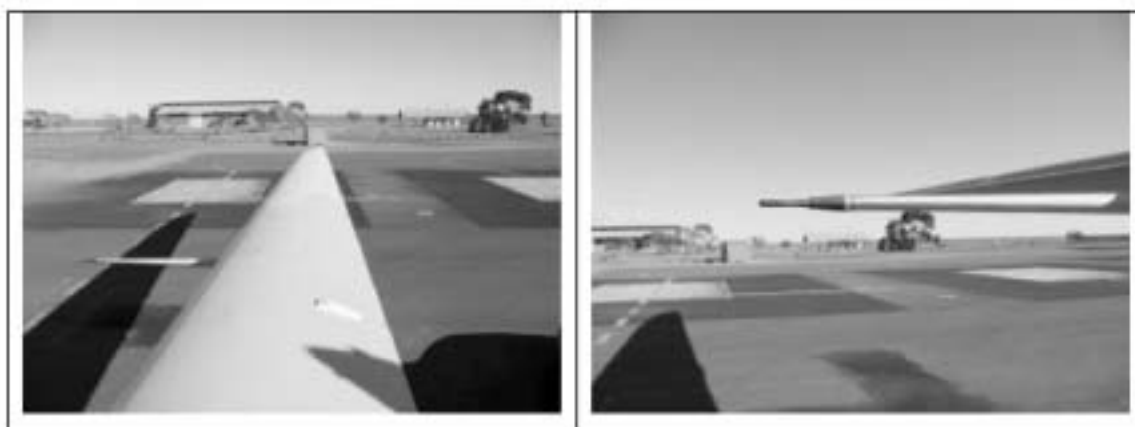
Figure 9: Rosemount 858 five-hole-probe mounted underneath the r/h wing of the Egrett
