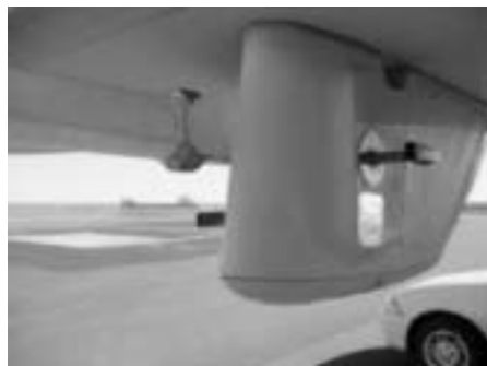
Figure 10: Rosemount 102 reverse flow Pt500 temperature sensor mounted on the pylon underneath the r/h wing.
