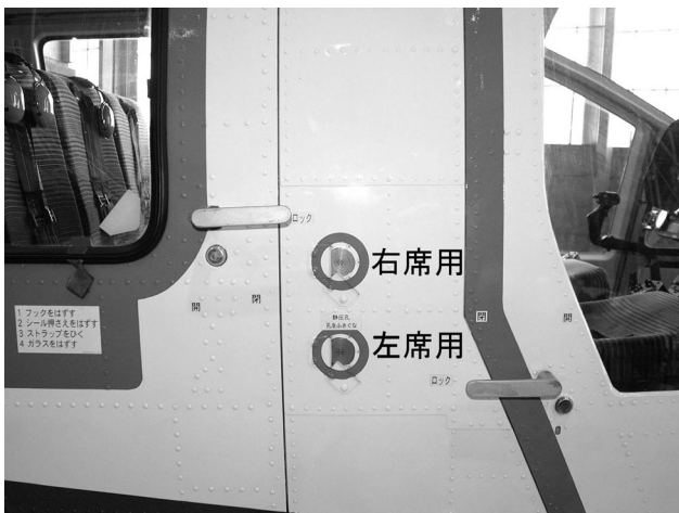
(c) 母機静圧孔 (右舷側, AERO INSTRUMENT ST 300-2 PT)
