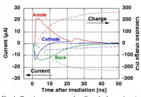
Fig. 4. Transient current and collected charge in n/n device when ion hits to the center area of p<sup>+</sup> region
