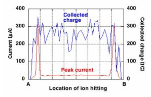
Fig. 3. Peak of transient current and total collected charge from anode electrode in n/n device as a function of the heavy ion hitting location
