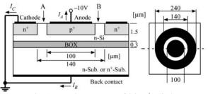
Fig. 1. Device structure of SOI  $p^+n$  diode
