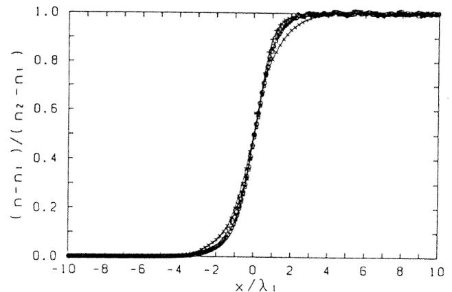
Fig. 3 Comparison of number density profile of shock wave;  $\circ$ , NC;  $\square$ , TC (present);  $\times$ , TC (Ref. 5);  $+$ , NMC (Ref. 6).
