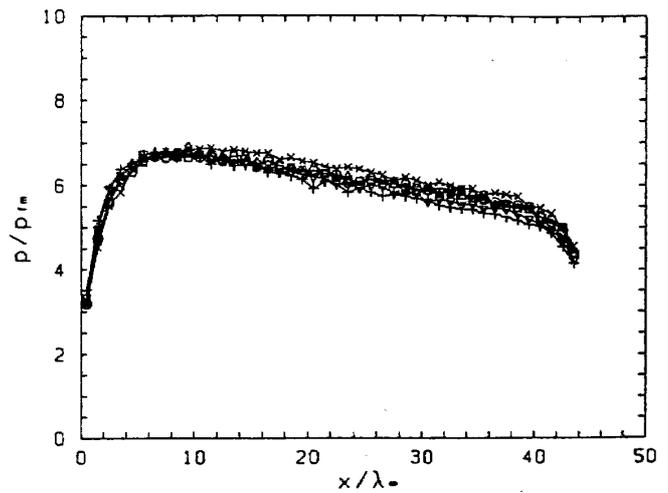
Fig. 5 Dependence of plate pressure distribution on the number of simulation molecule for the NC method;  $\circ$ ,  $N_0 = 7 \times 10^5$ ;  $\square$ ,  $N_0 = 5 \times 10^5$ ;  $\triangle$ ,  $N_0 = 3 \times 10^5$ ;  $\nabla$ ,  $N_0 = 10^5$ ;  $+$ ,  $N_0 = 5 \times 10^4$ ;  $\times$ ,  $N_0 = 10^4$ .
