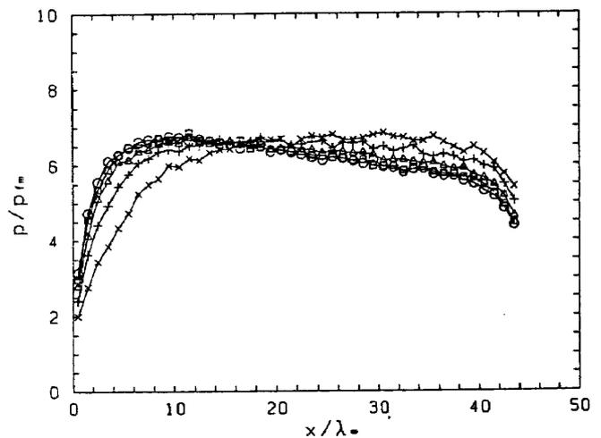
Fig. 6 Dependence of plate pressure distribution on the number of simulation molecule for the TC method;  $\circ$ ,  $N_0 = 7 \times 10^5$ ;  $\square$ ,  $N_0 = 5 \times 10^5$ ;  $\triangle$ ,  $N_0 = 3 \times 10^5$ ;  $+$ ,  $N_0 = 2 \times 10^5$ ;  $\times$ ,  $N_0 = 10^5$ .
