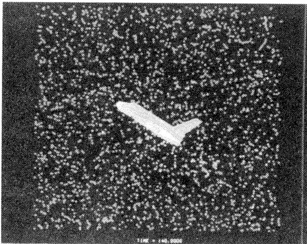
Fig. 1 Display of molecular positions around Shuttle-like plane.
