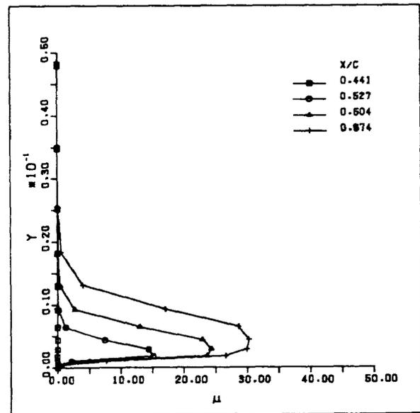
Fig. 3. Turbulent Viscosity Profiles (SHM):  $M_\infty = 0.8$ ,  $\alpha = 0$  and  $Re = 1 \times 10^6$ .
