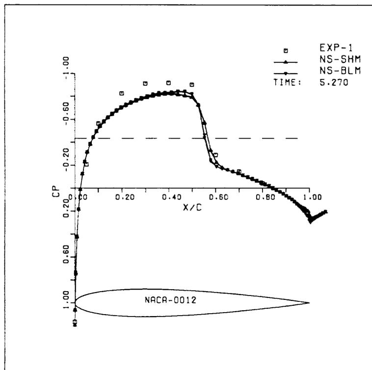
Fig. 6. Surface Pressure Distribution:
