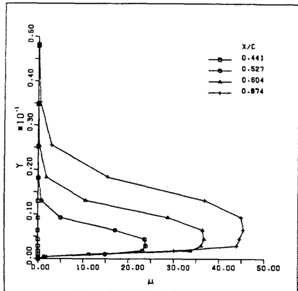
Fig. 2. Turbulent Viscosity Profiles (BLM):  $M_\infty = 0.8, \alpha = 0$  and  $Re = 1 \times 10^6$ .
