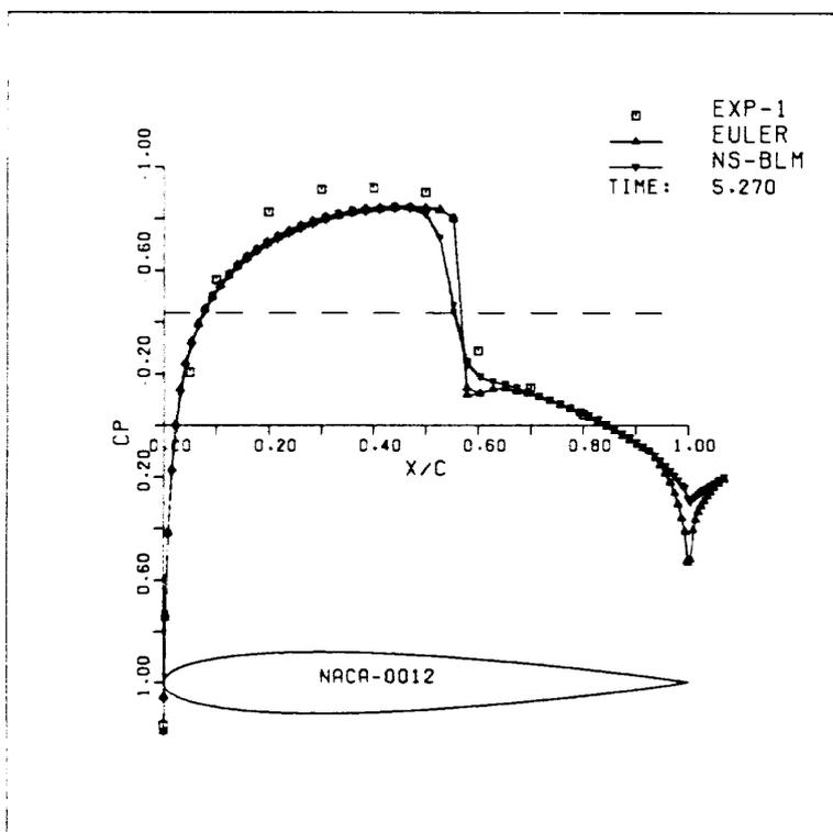
Fig. 5. Surface Pressure Distribution:
