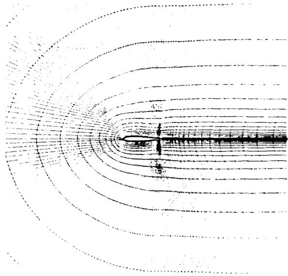
Fig. 1. 201 X 30 "C" Grid for NACA-0012 Airfoil
