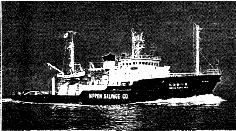
(a) Ship telemetry station and its antenna The ship whose name is DAINI-SEIHA-MARU(2nd calm-wave) is about 1000 gross tonnage. Four 5-elements cross-Yagi-antenna were installed.
