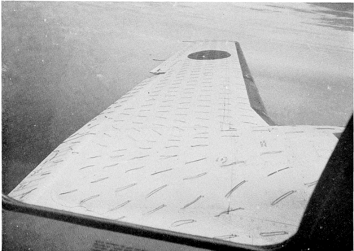
② POWER ON, GEAR UP, \delta_f = 11^\circ
