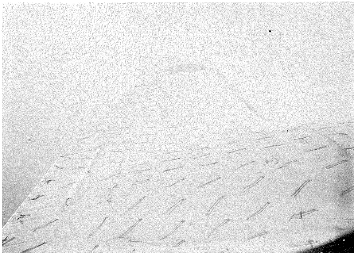
① POWER OFF, GEAR UP, \delta_f = 0^\circ
