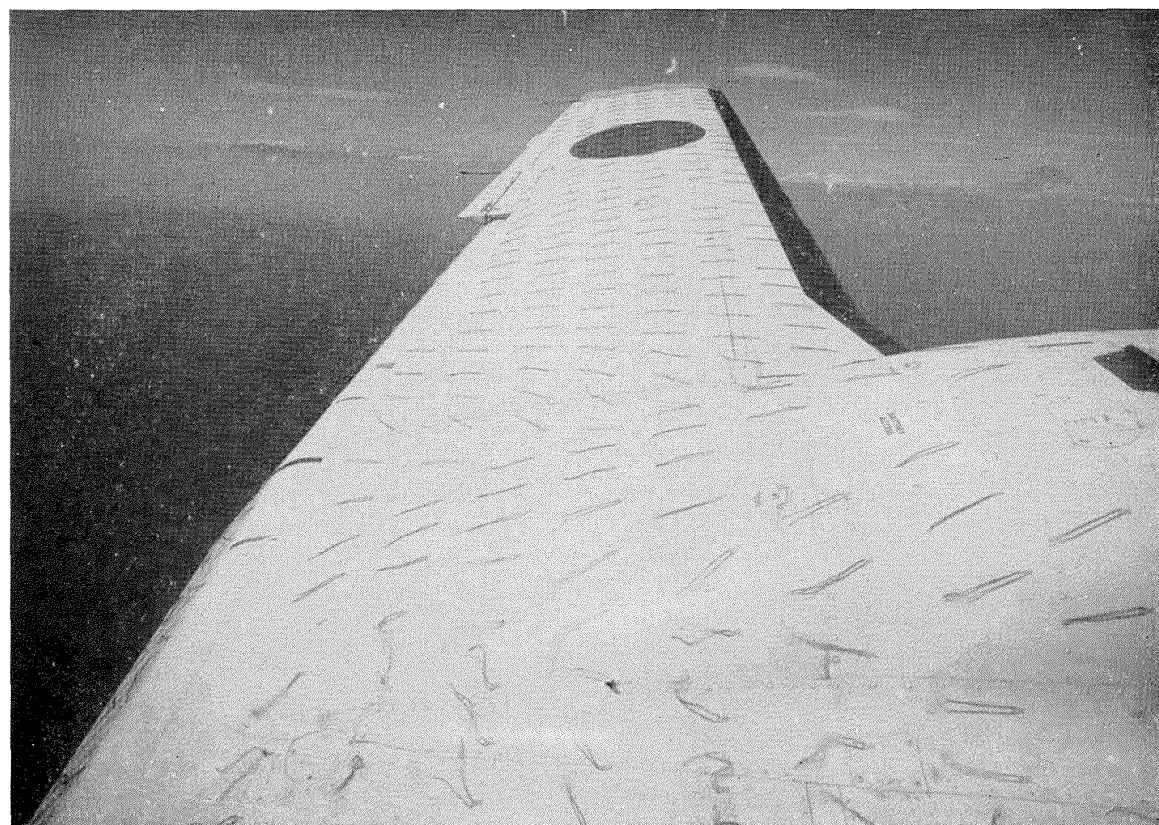
② POWER ON, GEAR DOWN, \delta_f = 28^\circ
