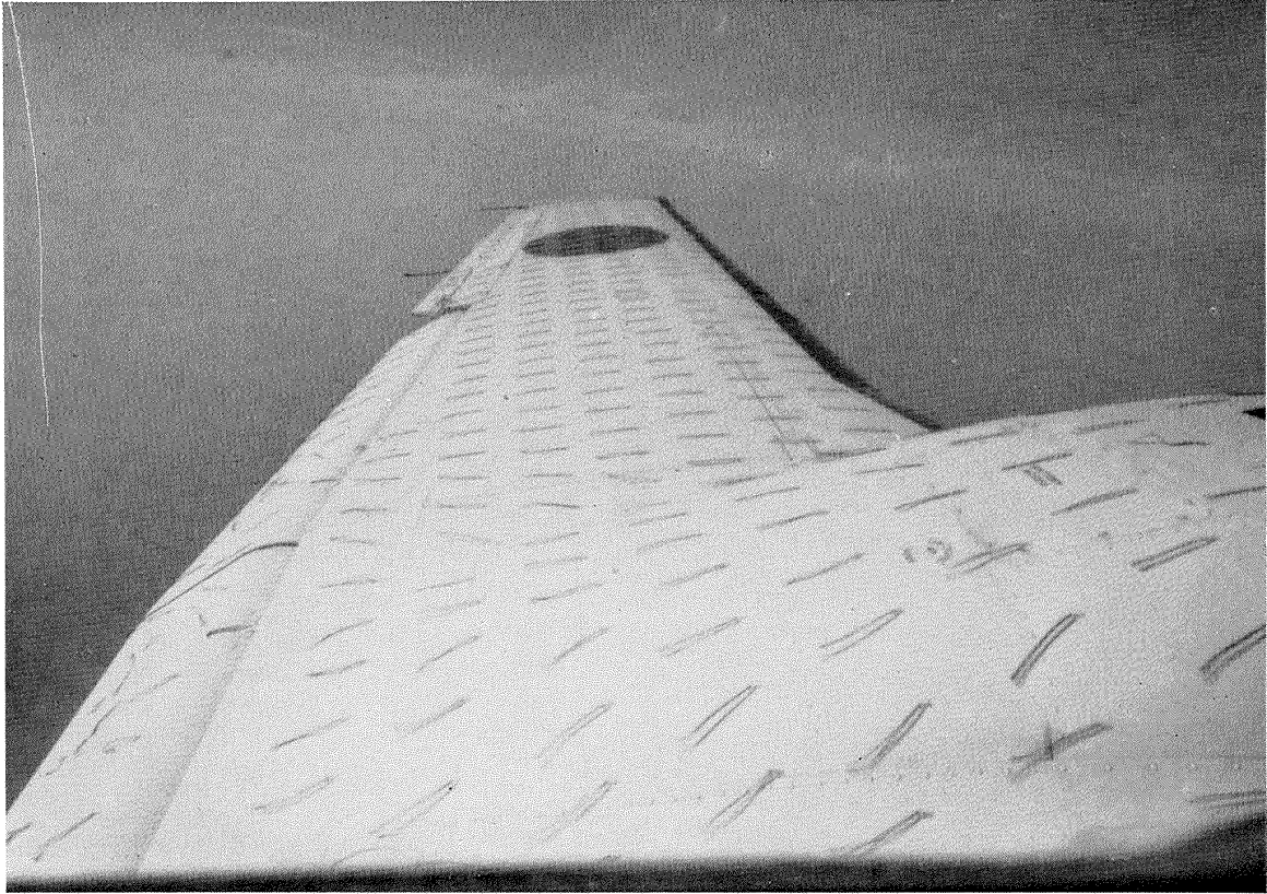
① POWER ON, GEAR DOWN, \delta_f=17^\circ
