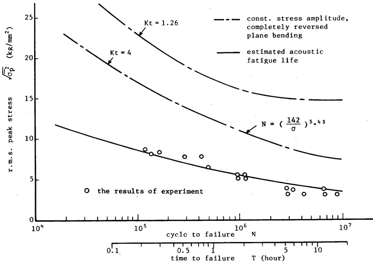
Fig. 10. Estimated S-N curve and experimental results.
