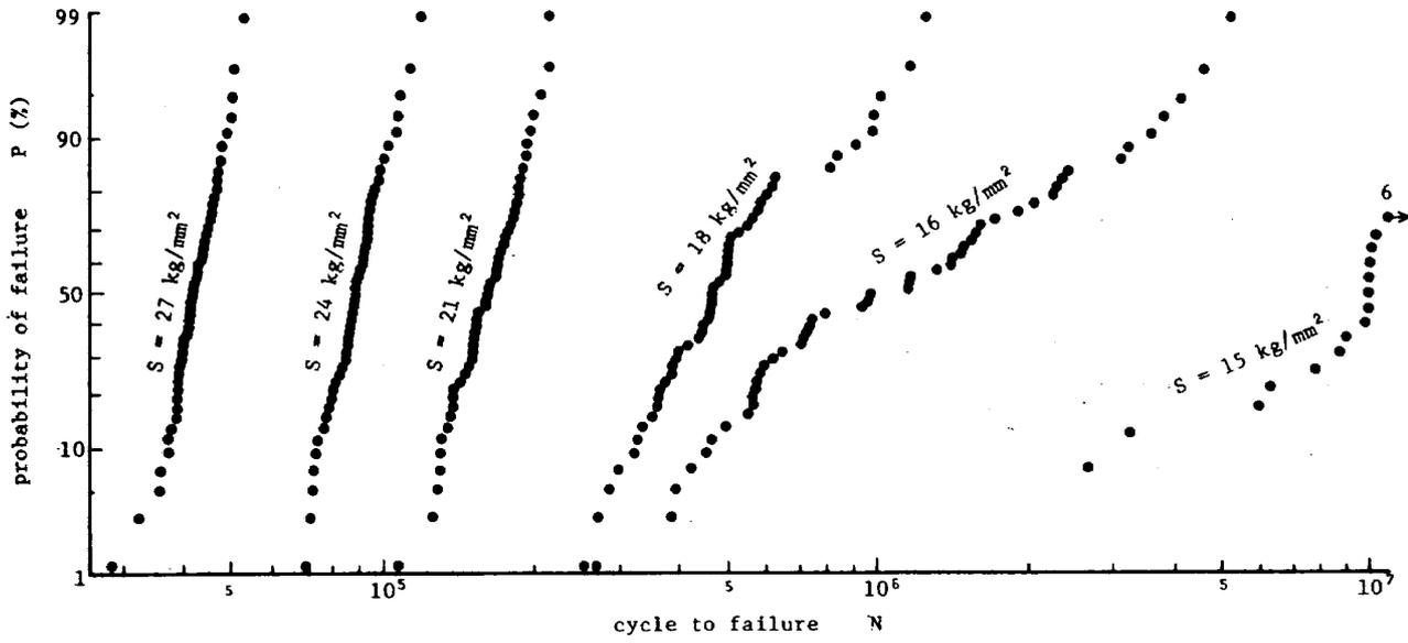
Fig. 5. Fatigue life distribution obtained by experiment.
