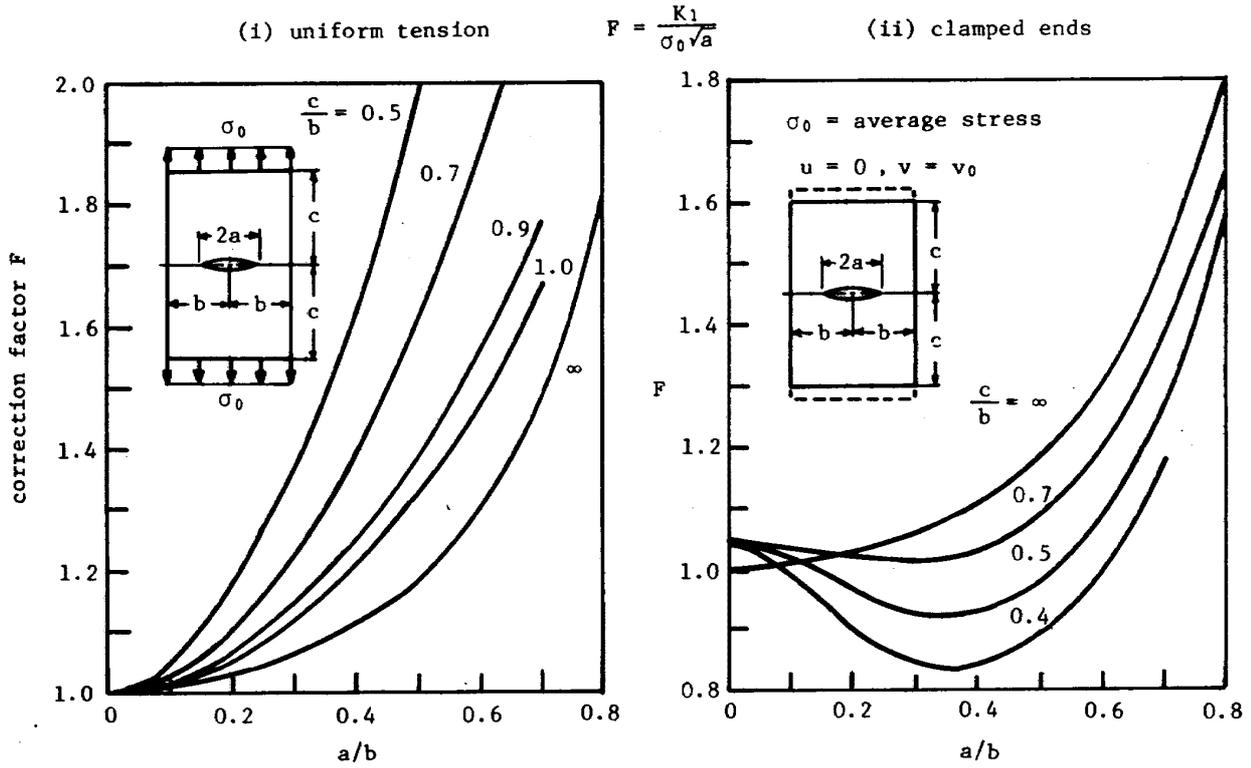
Fig. 9. Correction factors of  $K_1$  for uniform tension and clamped ends condition.
