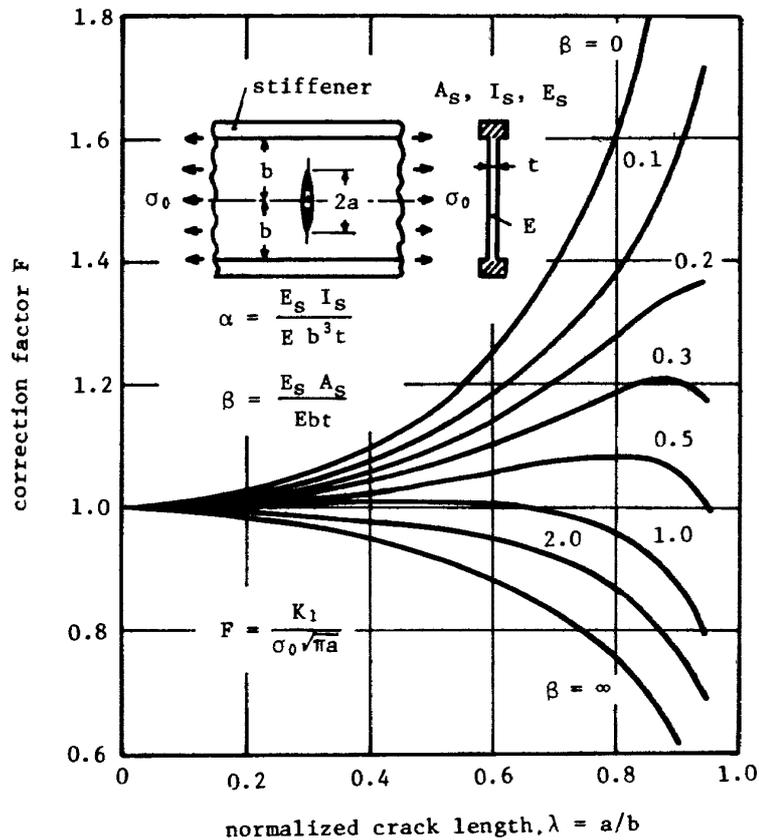
Fig. 8. Correction factor of  $K_1$  for  $\alpha=0.05$
