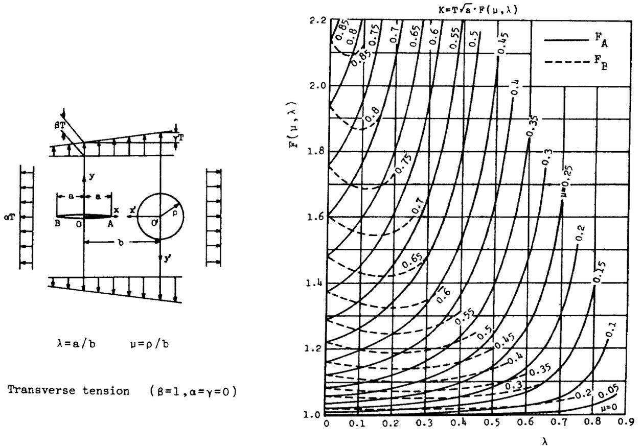
Fig. 7. Correction factor values for the crack approaching a hole.
