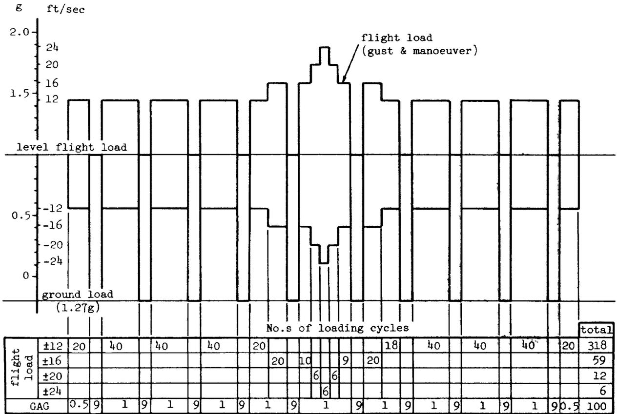
Fig. 11. Fatigue test spectrum of YS-11 full scale wing (for 100 flights).
