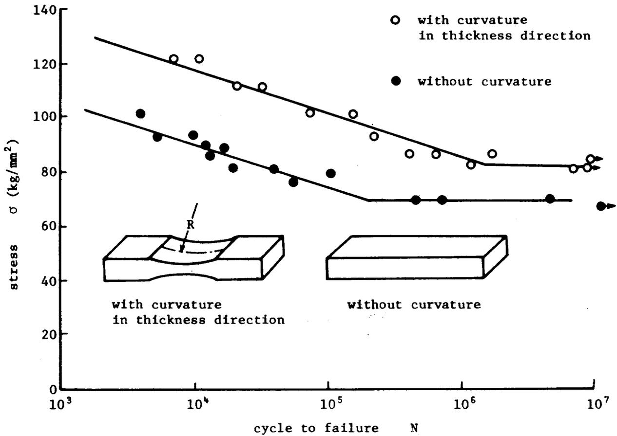
Fig. 6. S-N curve for CFRP.
