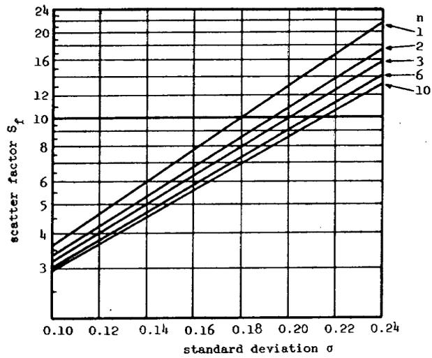
Fig. 13. Scatter factors ( $S_f$ ) for  $P=10^{-5}$  ( $k_p=4.26$ ) and  $1-\beta=0.90$  ( $k_\beta=1.26$ ).
