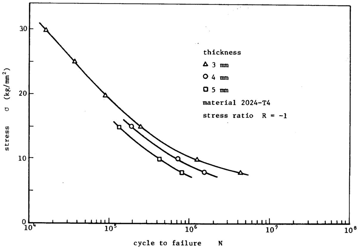
Fig. 4. Influence of specimen thickness.
