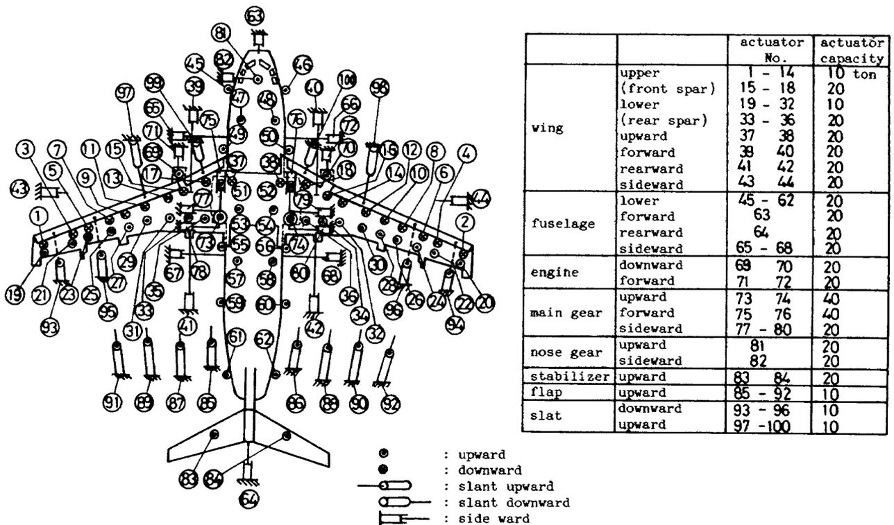
Fig. 12. Actuator arrangement of C-1 full scale fatigue test.
