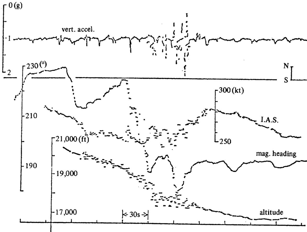
Fig. 4 Records of severe turbulence, Event No. 4
