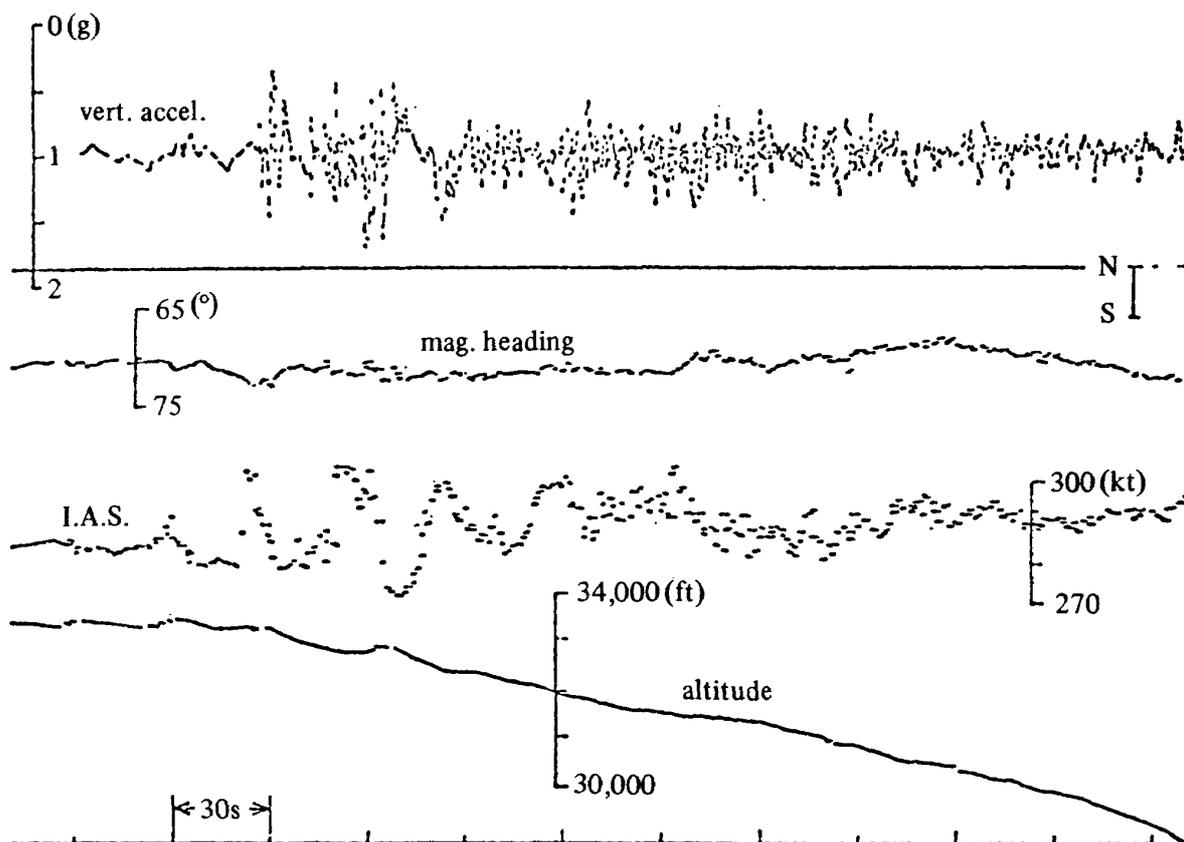
Fig. 5 Records of severe turbulence, Event No. 6
