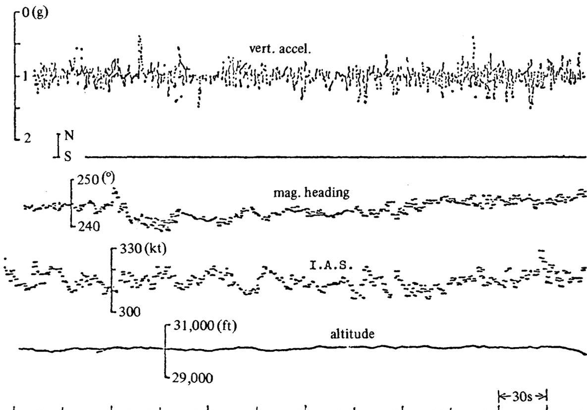
Fig. 2 Records of severe turbulence, Event No.2
