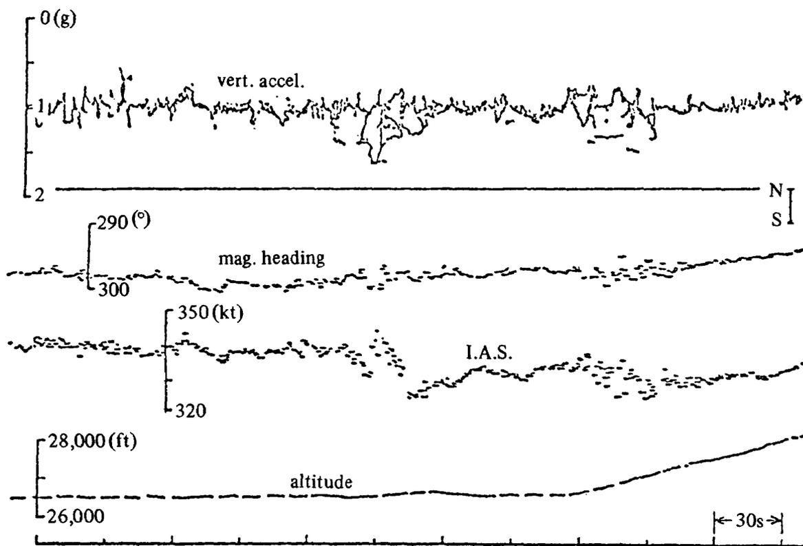
Fig. 3 Records of severe turbulence, Event No. 3
