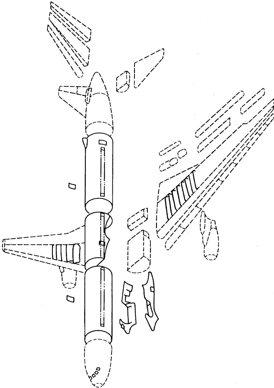
Fig. 23 Work Packages Allocated to Japan in the Development of Boeing 767
