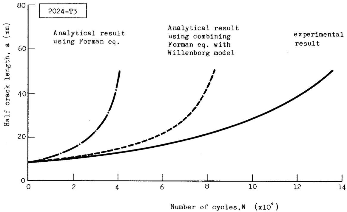
Fig. 20 An Example of a-N Curve Comparison between Analytical and Experimental Results Tested by Flight-by-Flight Program
