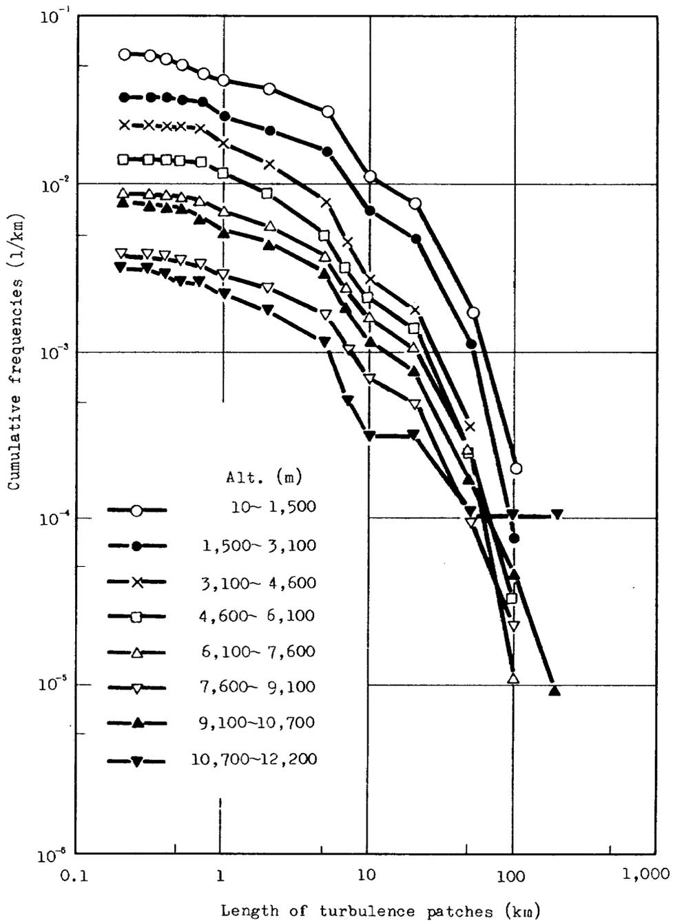
Fig. 3 Frequencies Distributions of the Length of Turbulence Patches
