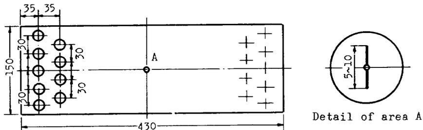
Fig. 6 The Center-cracked Strip Specimen
