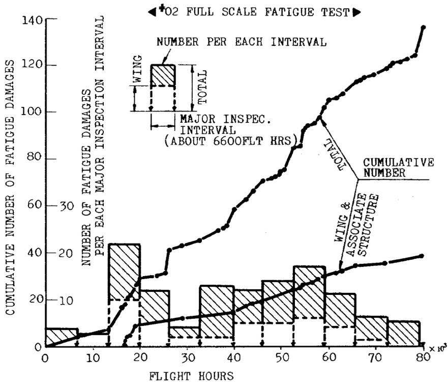
Fig. 28 Occurrence of Fatigue Damages
