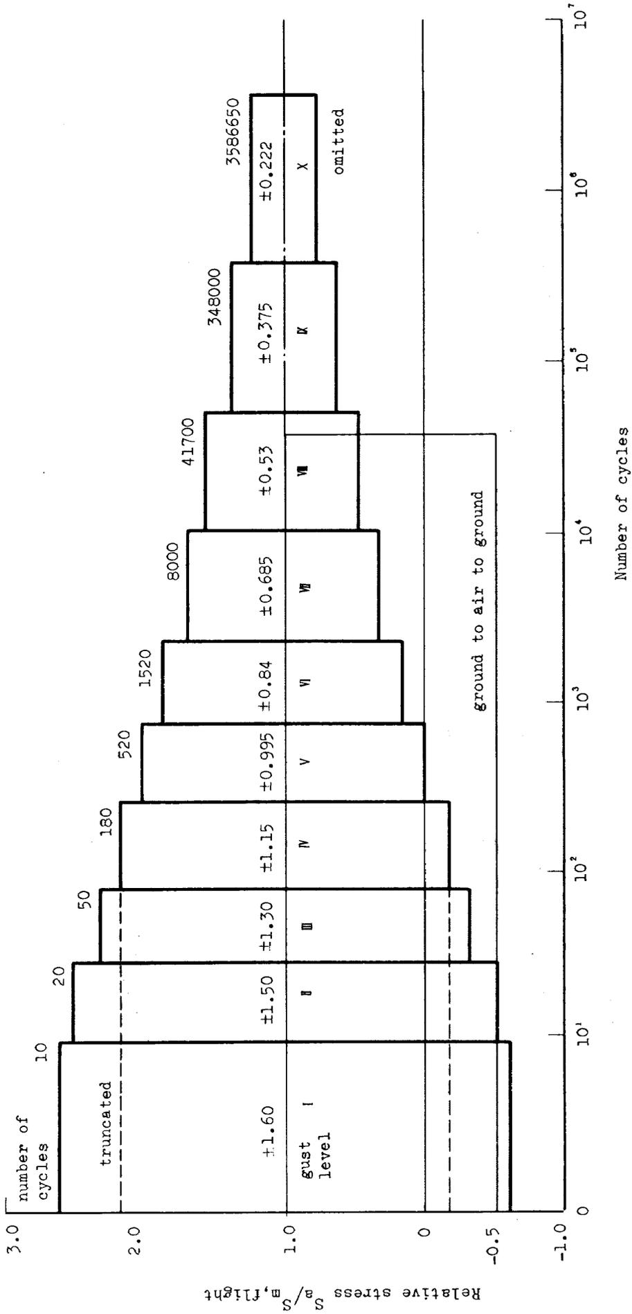
Fig. 10 Test Load Spectrum for 40,000 Flights
