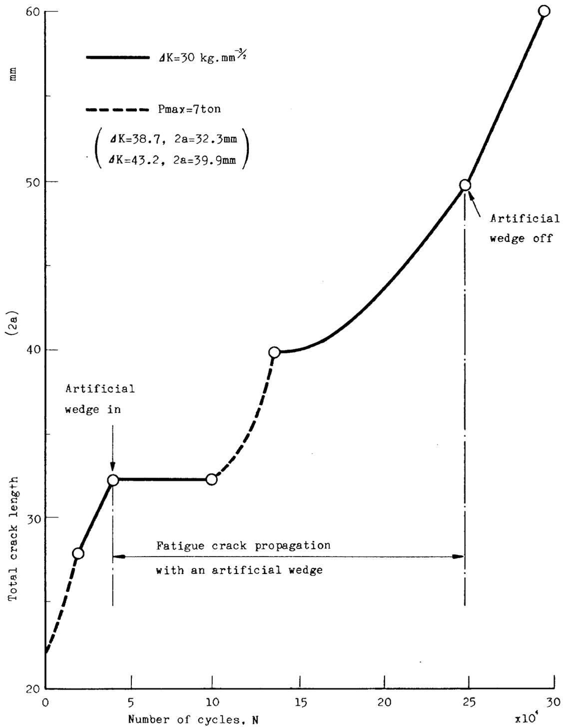
Fig. 22 An a-N Curve by a Fatigue Crack Propagation Test with and without an Artificial Wedge in the Crack
