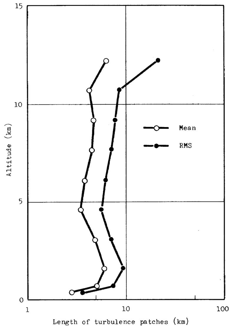
Fig. 4 Variation of the Length of Turbulence Patches with Altitude
