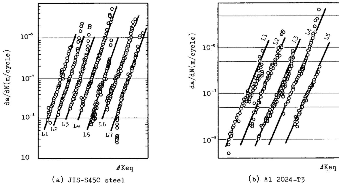
Fig. 8 Prediction of Crack Growth Rates by the HL Method
