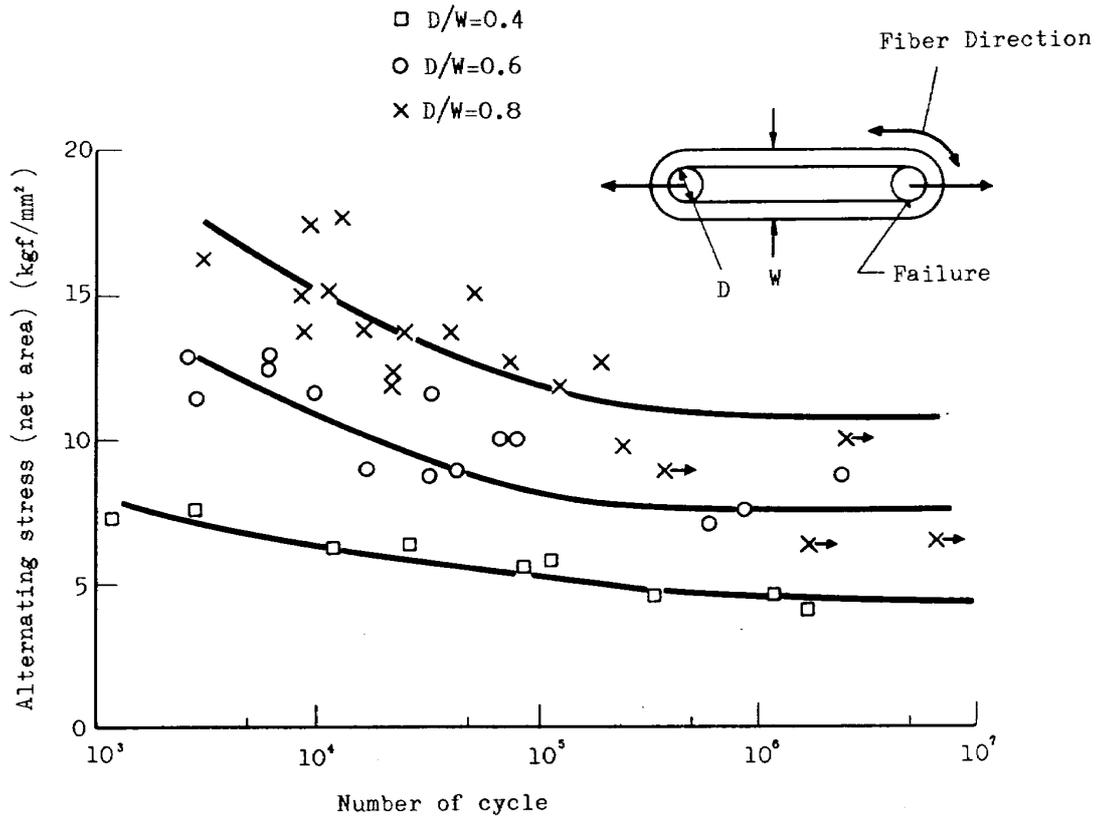
Fig. 29 Test Results of GFRP Lugs
