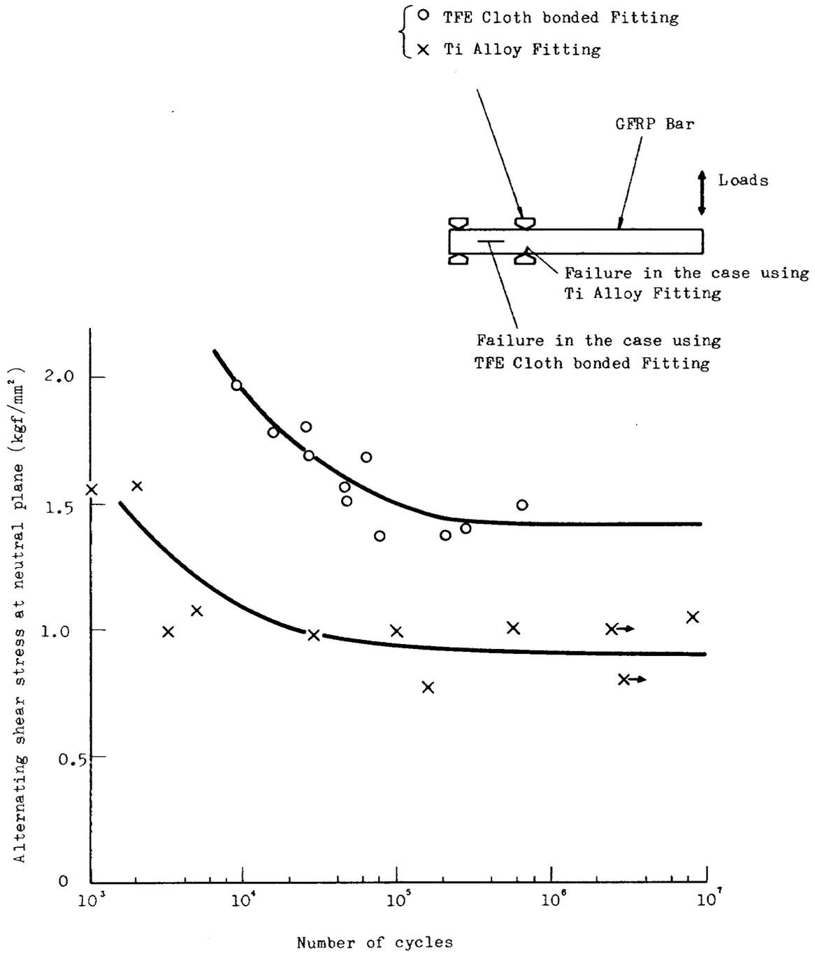
Fig. 31 S-N Curves for Surface Strength of GFRP Bars
