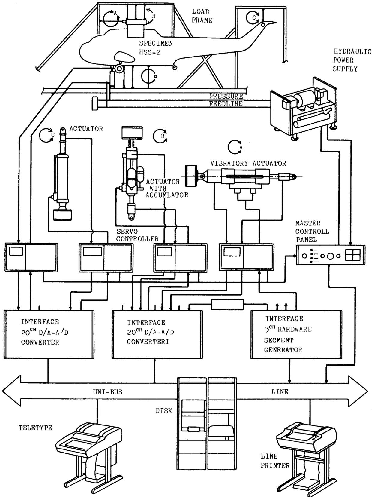
Fig. 21 Vibration Fatigue Testing System Scheme
