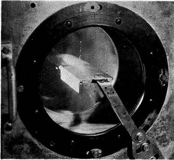
Fig. 1 Airfoil-flap combination model for Experiment 1
