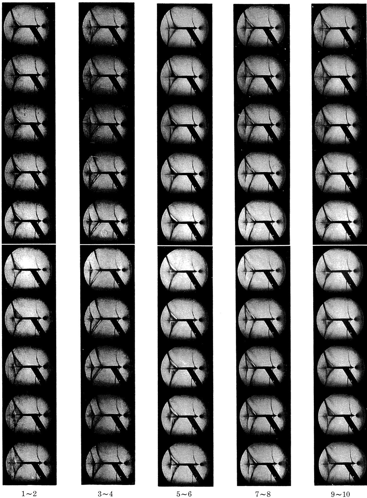
Fig. 9 Buzz oscillation at  $M=1.04$  Steel flap Incidence  $0^\circ$
