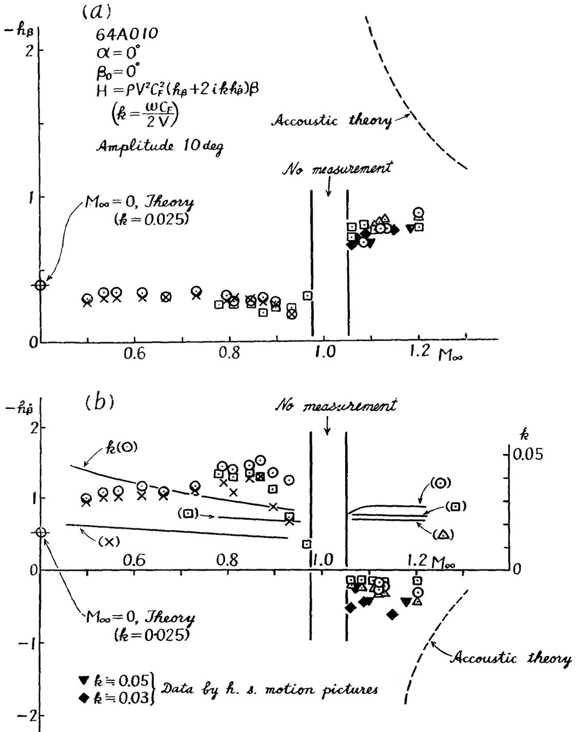
Fig. 10 Unsteady hinge moment coefficients of the flap at subsonic and transonic Mach numbers
