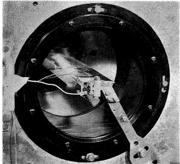
Fig. 2 Airfoil-flap combination model for Experiment 2
