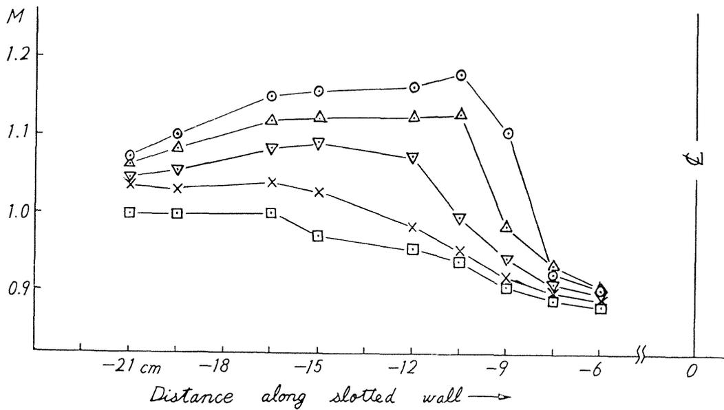
Fig. 3 Mach number distributions along roof slotted wall
