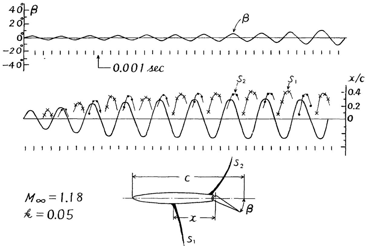
Fig. 6 Wave forms of flap angle and locations of shock waves during the growth of buzz
