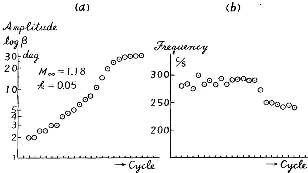
Fig. 7 Variations of amplitude and frequency during the growth of buzz
