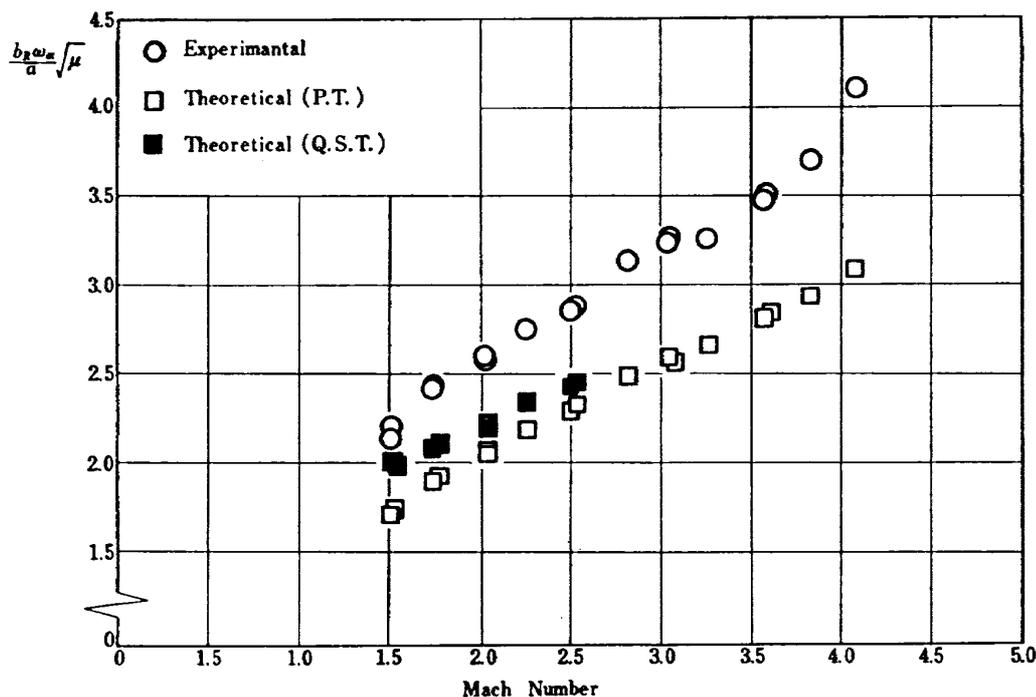
Fig. 4 Experimental and Theoretical Variaton of Stiffness-Altitude Parameter with Mach Number.
