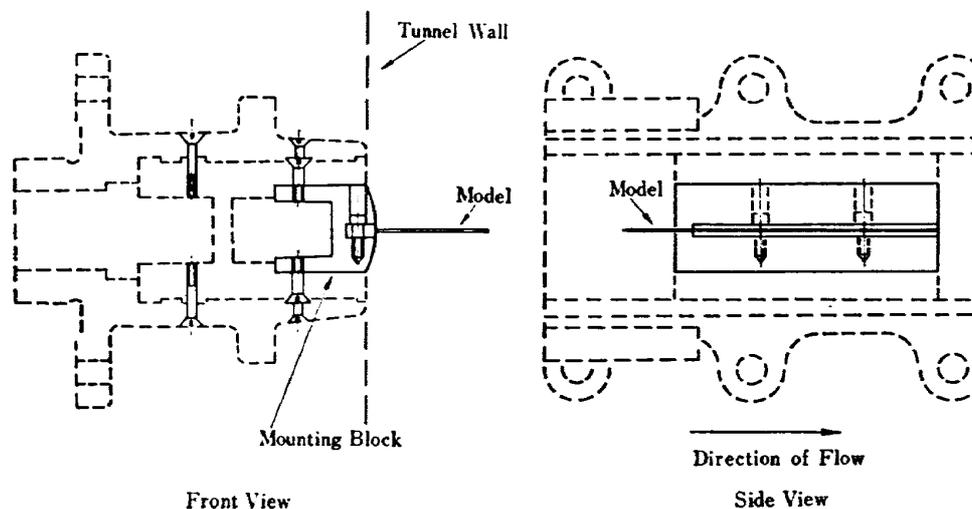
Fig. 2 Method of Mounting Model
