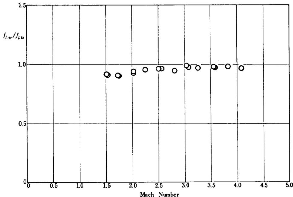
Fig. 5 Variation of the Ratio of Experimental to Theoretical Flutter Frequency with Mach Number.
