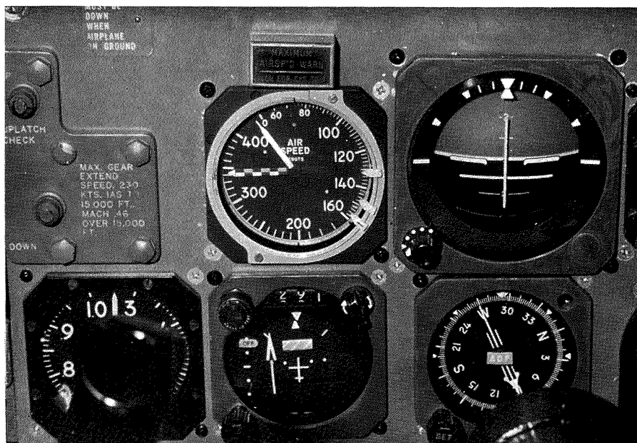
Fig. 8. Outlook of HFDI and PDI Upper Right: Horizontal Flight Director Indicator Center Bottom: Pictorial Deviation Indicator
