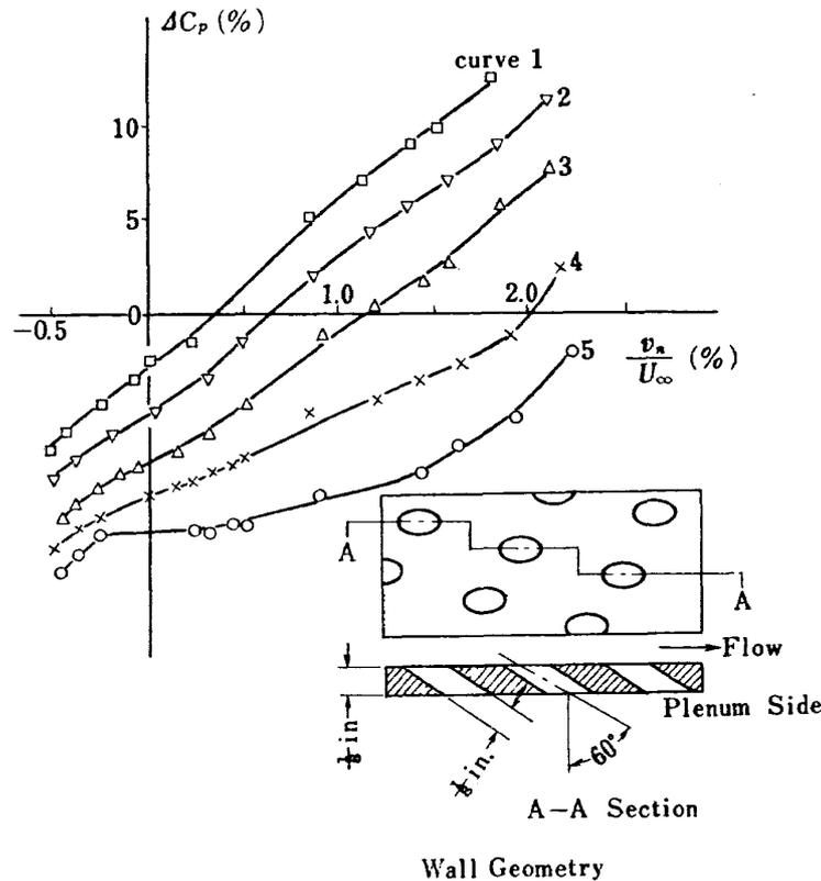
Fig. 5 Perforated Wall Characteristics for Various Boundary Layer Thicknesses (reproduced from ref. 26)
