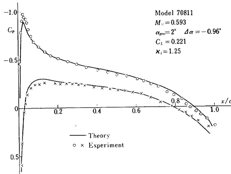
Fig. 8 (b) Pressure Distributions on Model 70811,  $M_\infty = 0.6$ ,  $\alpha = 2^\circ$
