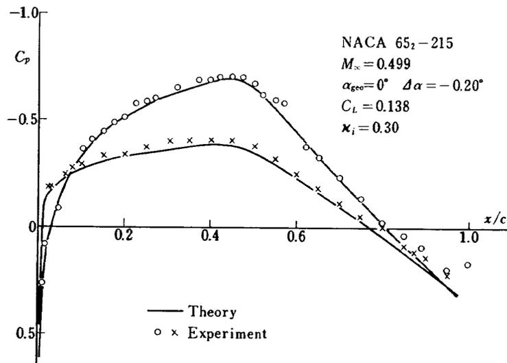
Fig. 9 (a) Pressure Distributions on the NACA 65<sub>2</sub>-215 Model,  $M_\infty = 0.5, \alpha = 0^\circ$
