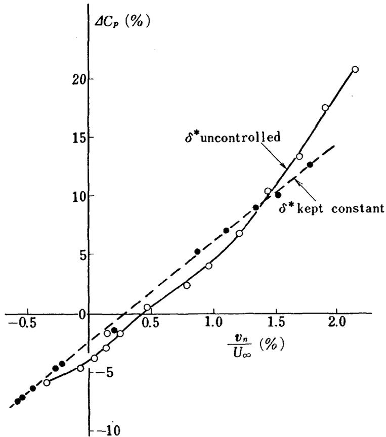
Fig. 4 Comparison of Perforated Wall Characteristics Determined under Constant and Variable Boundary Layer Thicknesses (reproduced from ref. 26)
