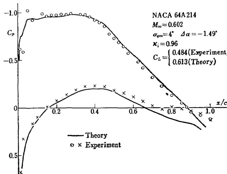
Fig. 10 (b) Pressure Distributions on the NACA 64A214 Model,  $M_\infty=0.6, \alpha=4^\circ$
