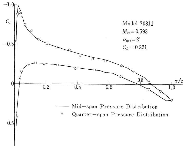
Fig. 7 Two-dimensionality of the Test Data
