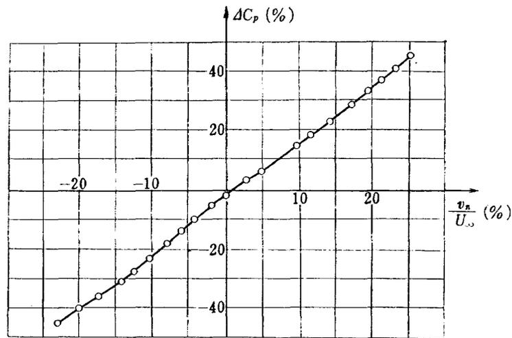
Fig. 1 Characteristics of a 1-inch Transverse Slot (reproduced from refs. 21 & 22)
