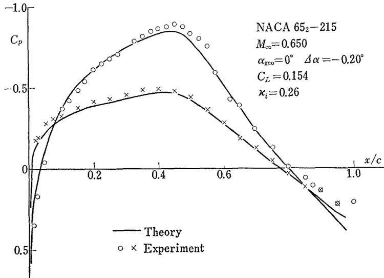
Fig. 9 (c) Pressure Distributions on the NACA 65<sub>2</sub>-215 Model,  $M_{\infty}=0.65, \alpha=0^{\circ}$
