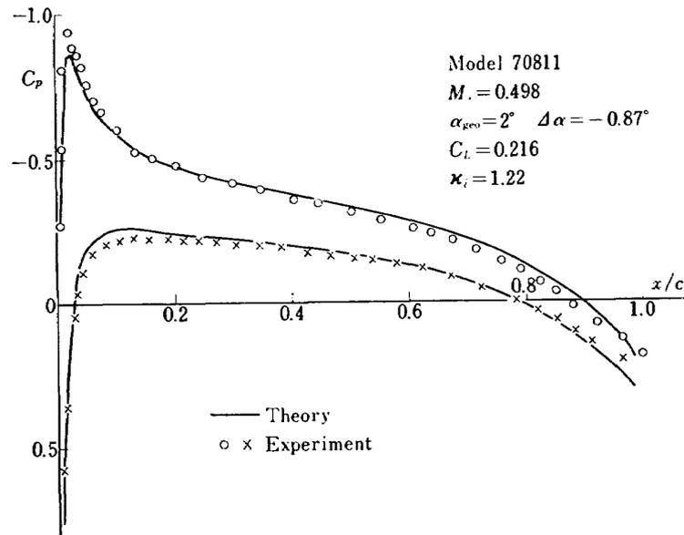
Fig. 8 (a) Pressure Distributions on Model 70811,  $M_\infty = 0.5$ ,  $\alpha = 2^\circ$
