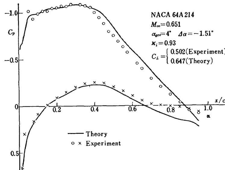
Fig. 10 (c) Pressure Distributions on the NACA 64A214 Model,  $M_\infty=0.65, \alpha=4^\circ$
