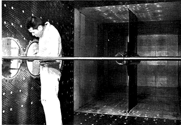
Fig. 6 The test section of the NAL 2m×2m wind tunnel with the Model 70811 installed
