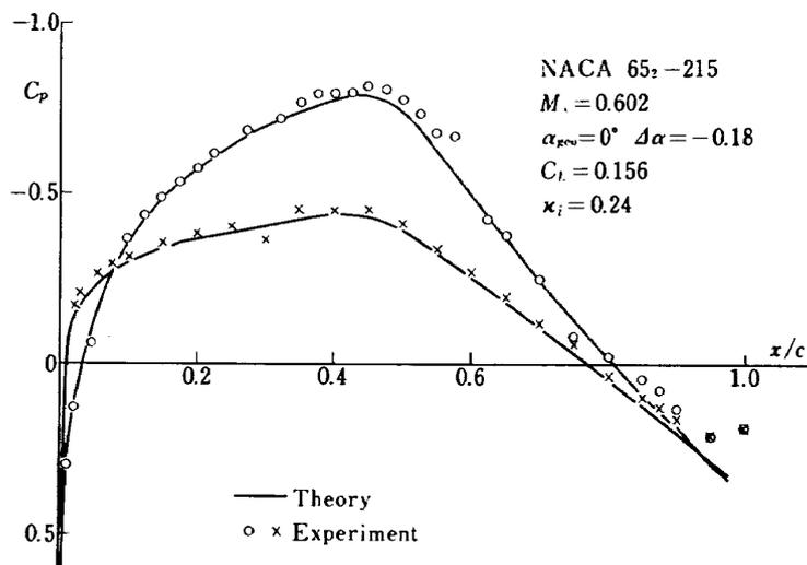
Fig. 9 (b) Pressure Distributions on the NACA 65<sub>2</sub>-215 Model,  $M_\infty = 0.6, \alpha = 0^\circ$
