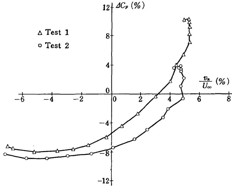
Fig. 3 Characteristics of Perforated Sheets under the Influence of an Aerofoil Model (reproduced from ref. 24)
