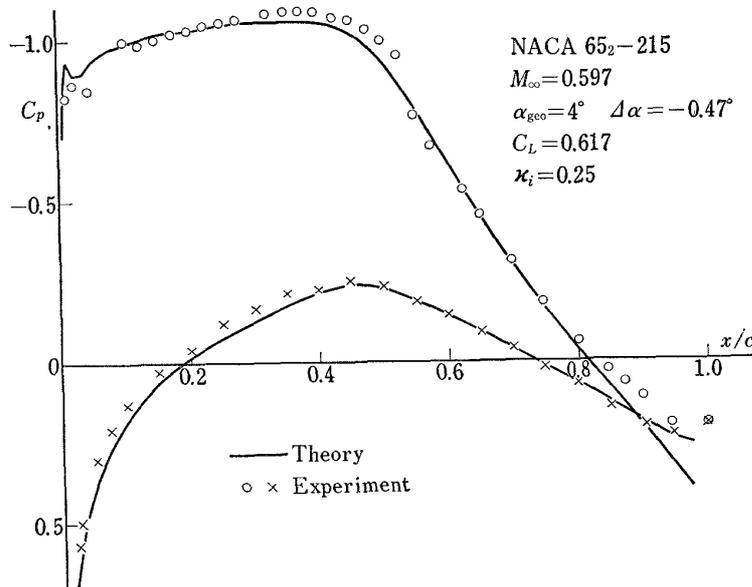
Fig. 9 (e) Pressure Distributions on the NACA 65<sub>2</sub>-215 Model,  $M_{\infty}=0.6, \alpha=4^{\circ}$
