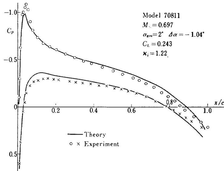
Fig. 8 (c) Pressure Distributions on Model 70811,  $M_\infty = 0.7, \alpha = 2^\circ$
