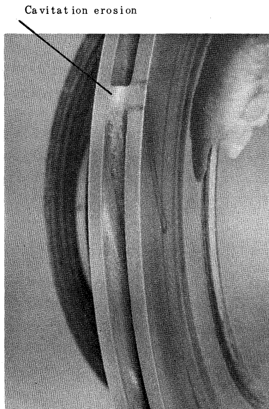
Fig. 5-15 Cavitation erosion at the tip of an impeller.
