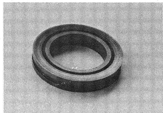
Fig. 5-29 Mechanical seal (After liquid nitrogen test).
