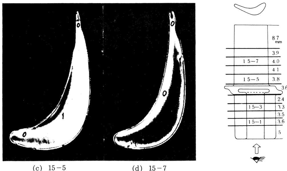
Fig. 17 Fringe pattern and fringe order distributions at lateral cross-sections of hollow turbine blade model
