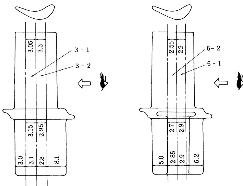
Fig. 13 Position of slice models in blades (Numerals in mm)
