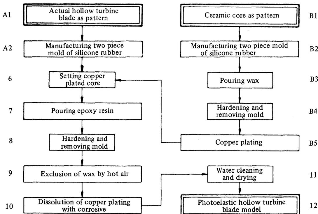
Fig. 1 Manufacturing procedure of three-dimensional hollow photoelastic models
