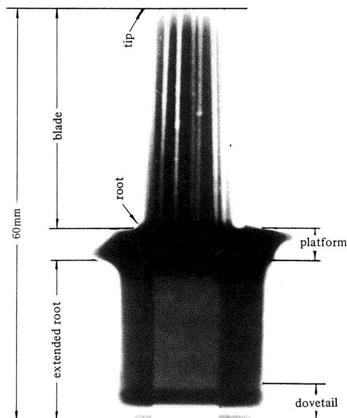
Fig. 4 X-ray photograph of actual turbine blade
