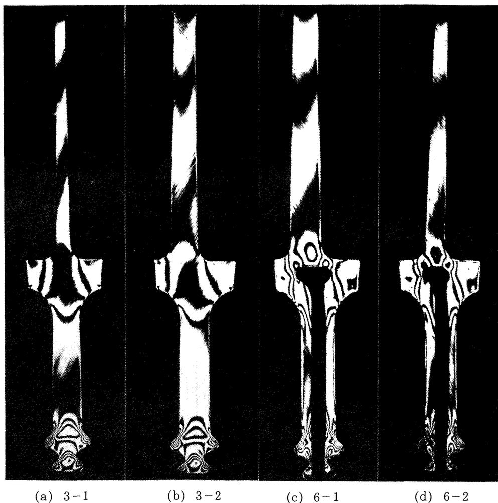
Fig. 12 Fringe patterns of sliced blade models
