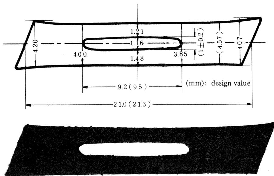
Fig. 3 A typical dimension of epoxy model
