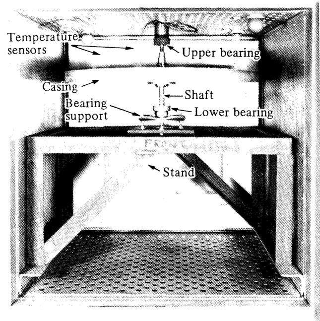
Fig. 6 Inside view of temperature controlled container with experimental rotating system
