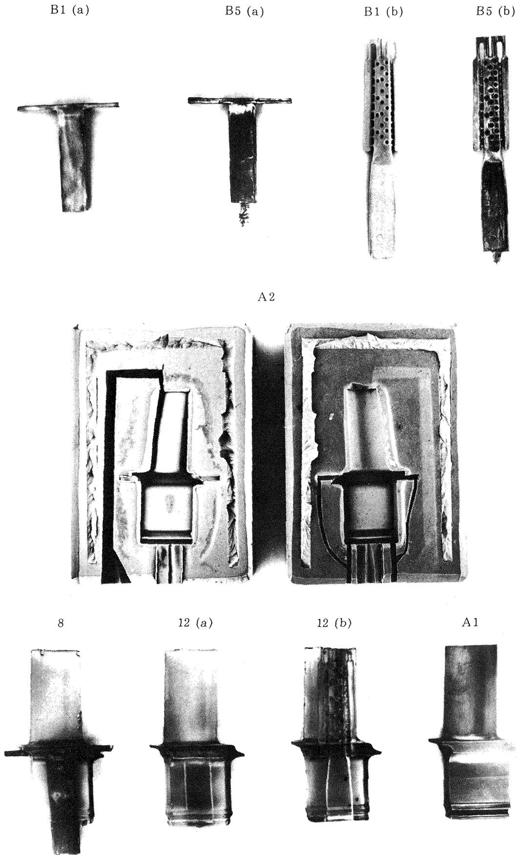
Fig. 2 Photographs at some manufacturing steps (Notation coincides with it in Fig. 1)
