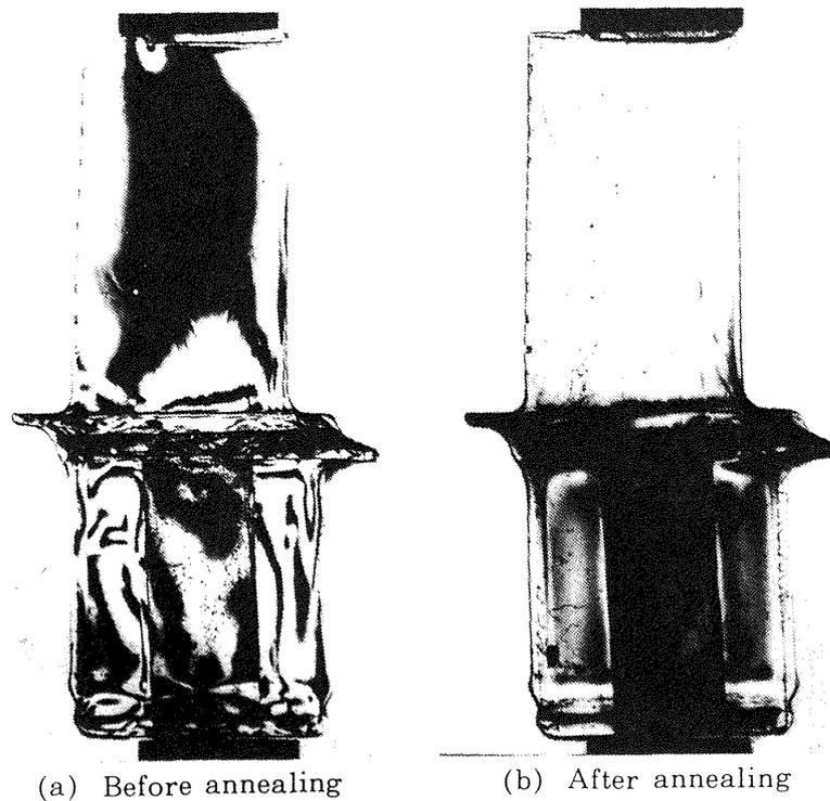
Fig. 9 Annealing condition of blade model
