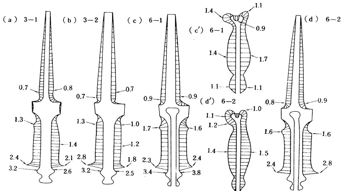
Fig. 15 Surface stress distributions on slice models (Numerals in fringe order/unit thickness)
