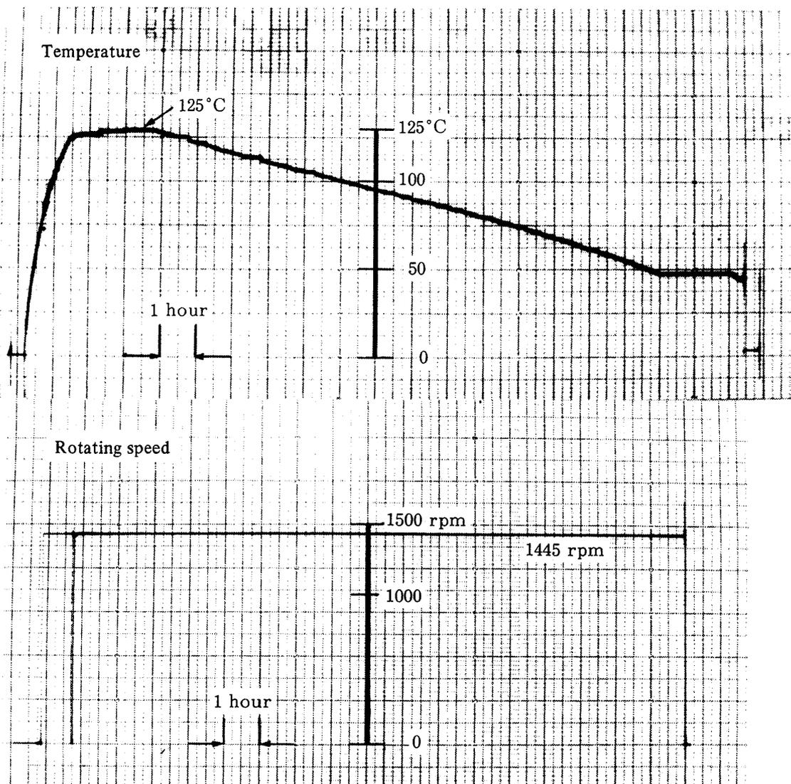
Fig. 8 Temperature and rotating speed variations in container during stress freezing
