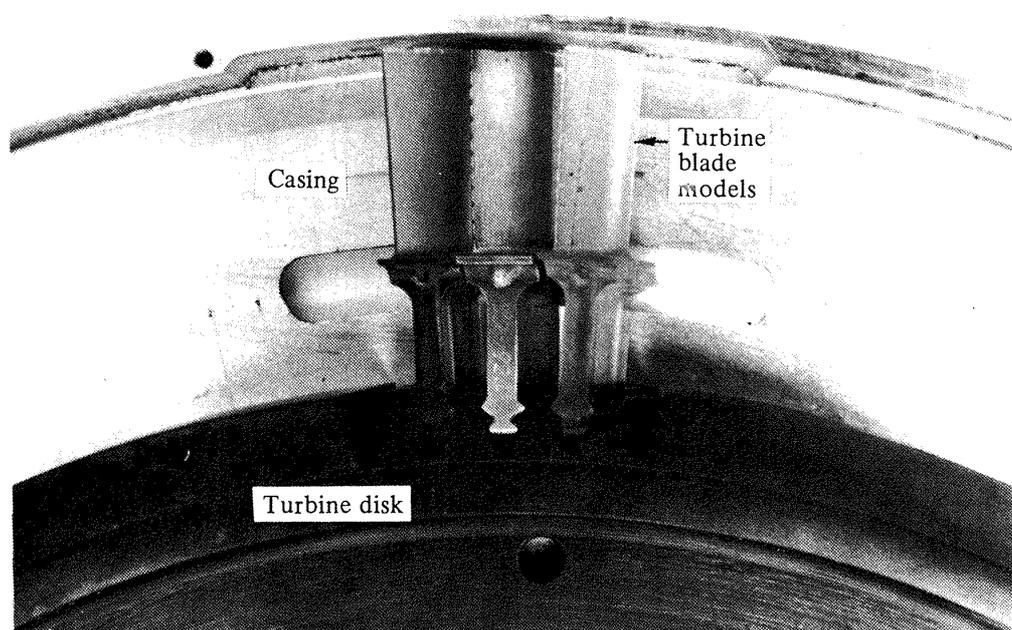
Fig. 7 Inside view of casing
