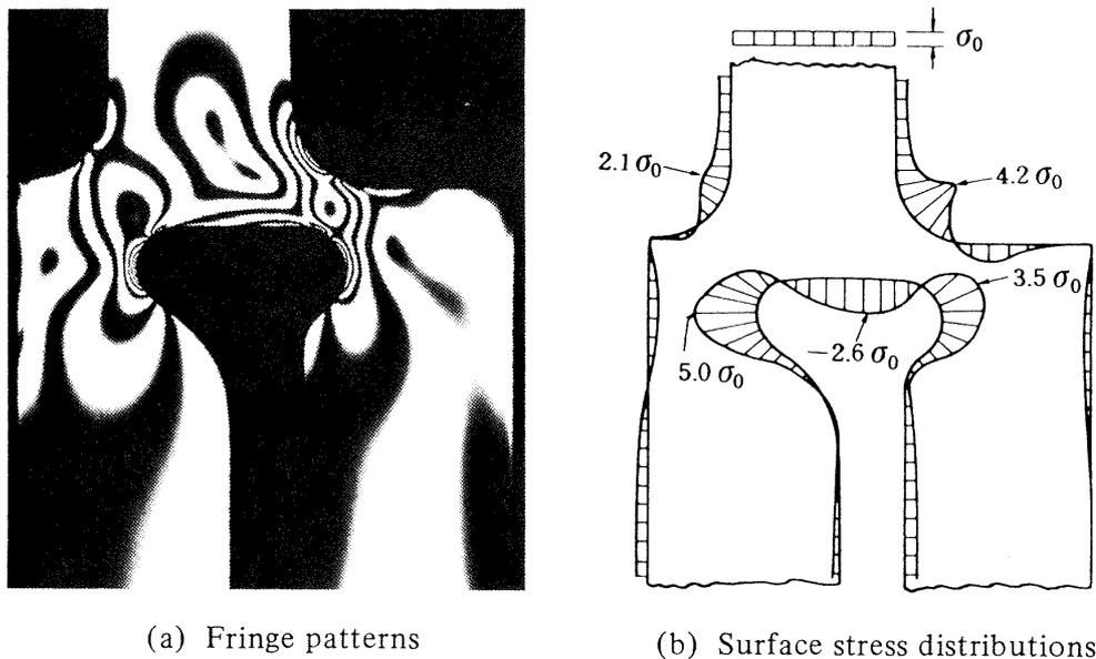
Fig. 16 Two-dimensional photoelastic test under tensile condition
