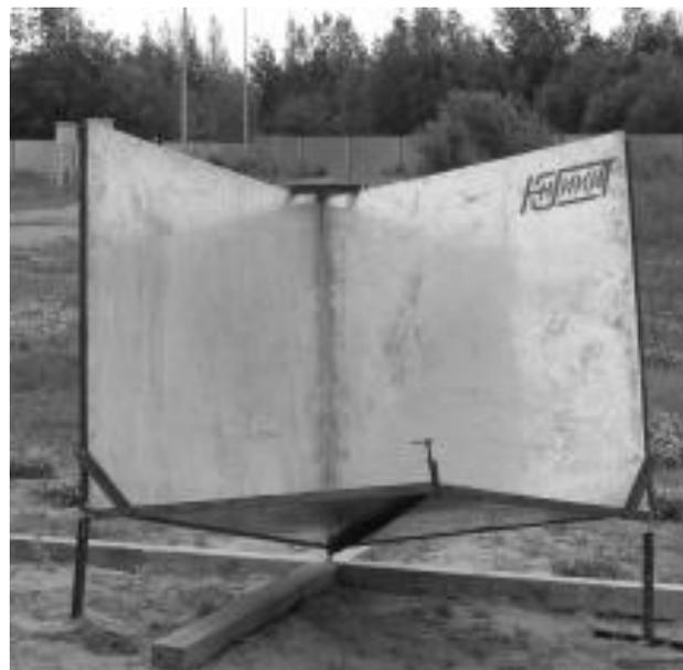
**Fig. 2 Trihedral corner reflector (1.25m) installed on the test site of the city of Khanty-Mansiysk and aimed on ALOS\PALSAR ascending acquisitions**
