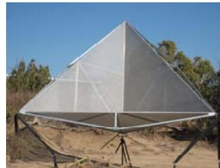
Fig. 3 One of the 2.4 m radar corner reflectors at Pinon Flat Observatory installed in 1998. This arid region at an elevation of 1200 m is relatively flat with a surface of decomposed granite sparsely covered by bush and grass. Three radar corner reflectors are oriented to reflect energy from ascending (A1) and descending (D1 and D2) ALOS passes.
