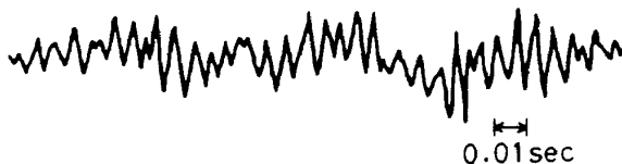
Fig. 2 A typical strain gauge signal at Q=78\% Q_f
