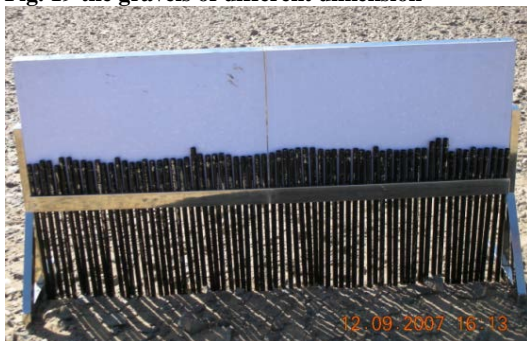
Fig. 20 the instrument for measuring surface roughness parameters
