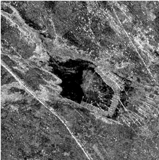
Fig.8 the detection result of the Great Wall in our study area based on SIR-C (L-HH)
