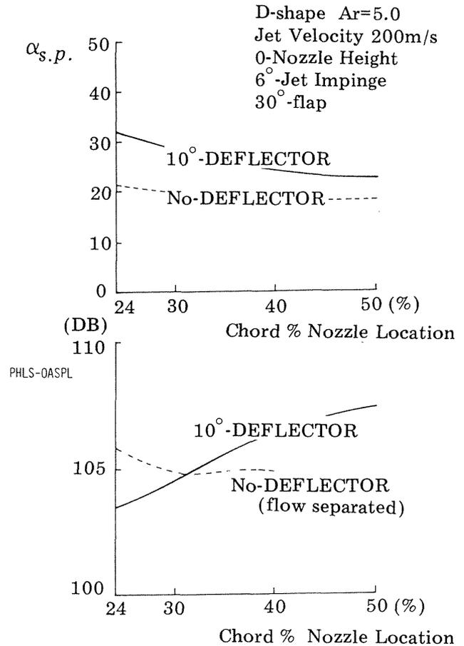
Figure 25 The effect of chordwise locations of USB nozzle on PHLs-OASPL and the parameter  $\alpha_{s.p.}$
