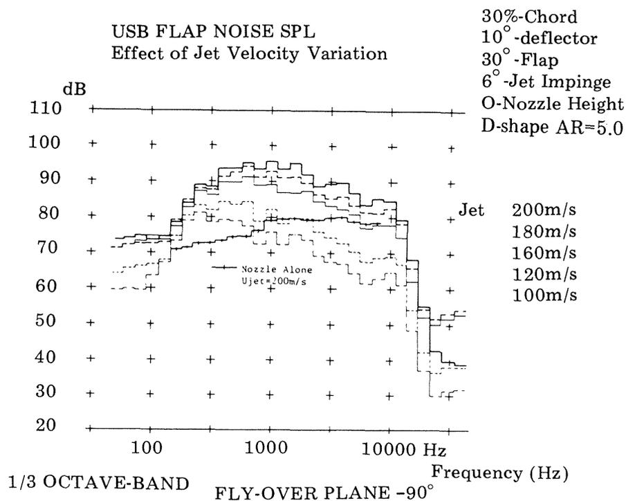
Figure 8 The effect of jet velocing variation on USB-PHLS noise spectra a at the direction below the wing (Flyover -90°)
