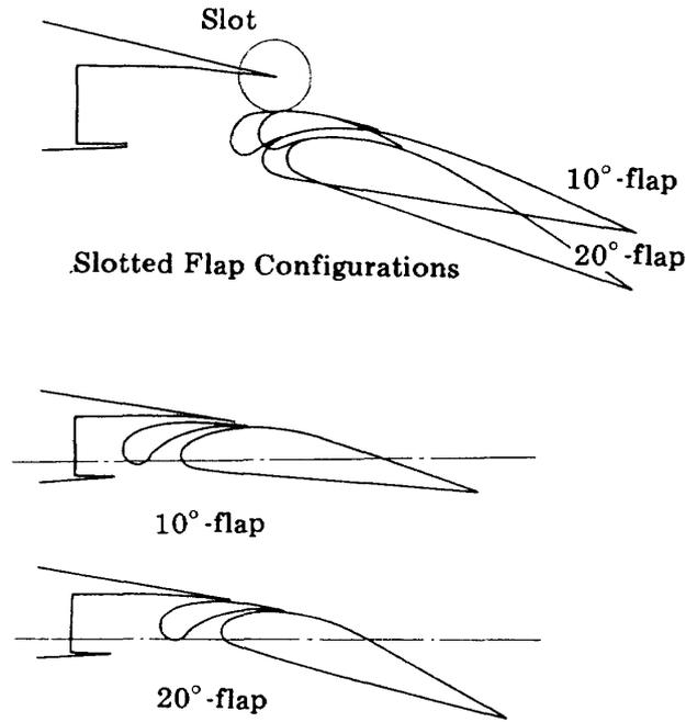
Figure 29-1 Slotted flap configuration being compared with basic double flap configurations (slot is 0.1% flap chord)
