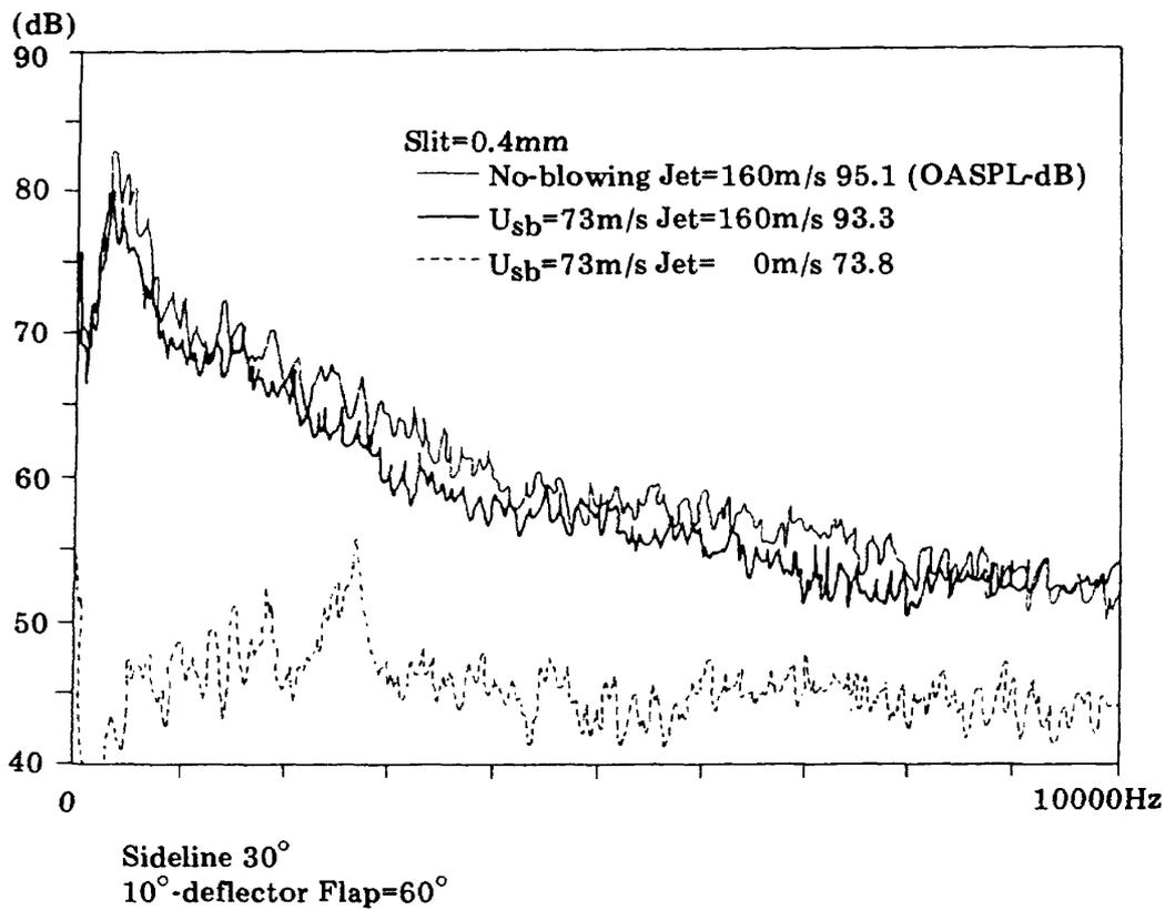
Figure 28-2 PHLs noise reduction by slit secondary blowing flap in narrow-band spectra
