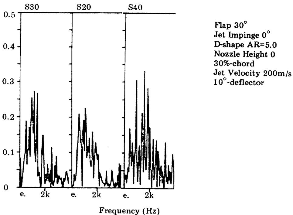
Figure 16 Coherence across flap trailing edge surface pressure at jet velocity 200m/s
