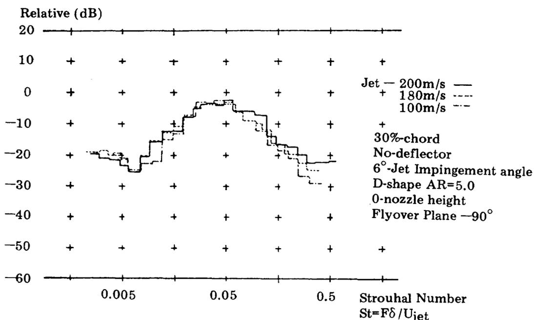
Figure 15 The normalized SPL spectral density using Strouhal number based upon the wall jet thickness at the flap trailing edge,  $\delta$
