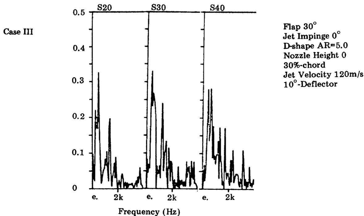
Figure 17 Coherence across flap trailing edge surface pressure at jet velocity 120m/s
