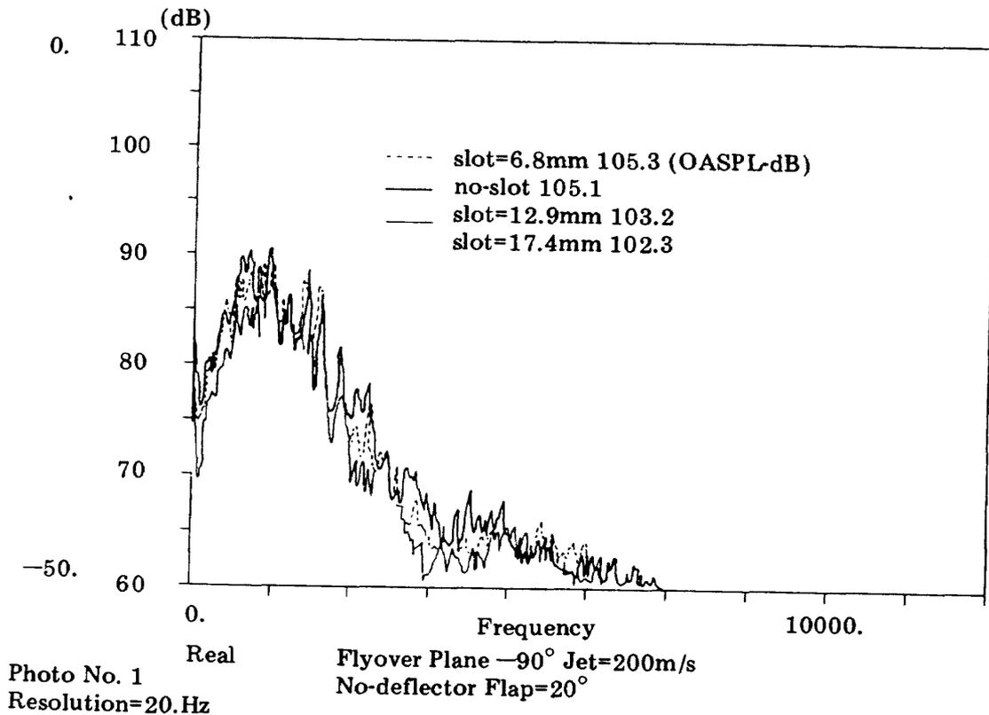
Figure 29-2 PHLs noise reduction by slotted flap
