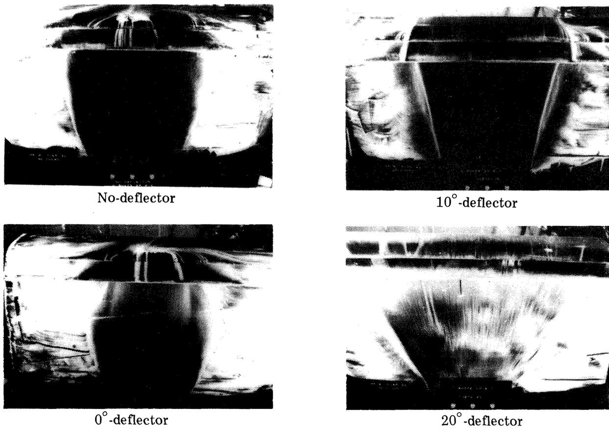
Figure 18-2 Flow visualization photographs by oil flows (Effect of Deflector type)
