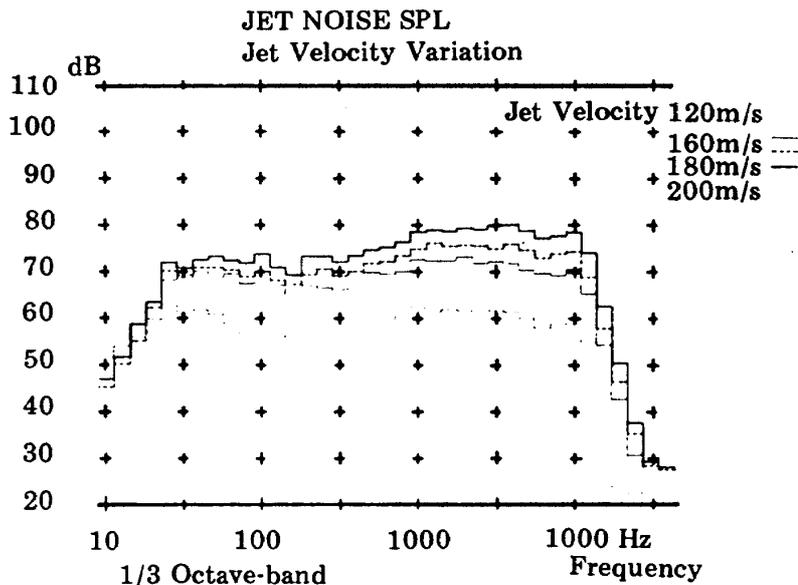
Figure 9 The effect of jet velocity variation on jet noise (Jet nozzle alone component case) at the direction below the wing (Flyover  $-90^\circ$ )
