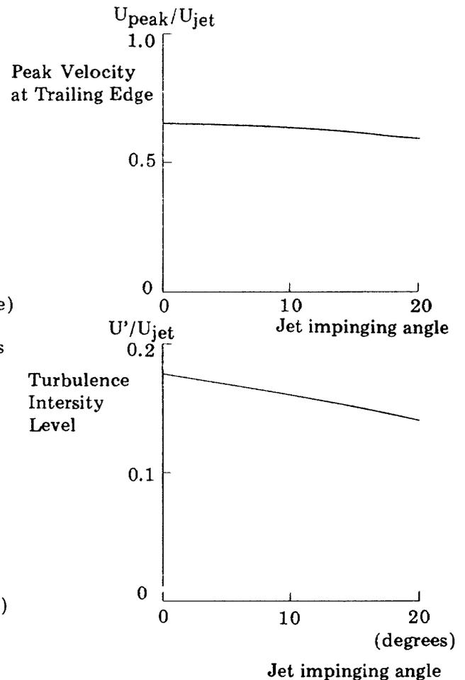
Figure 24 The effect of jet impingement angle variation on peak velocity and turbulence intensity level at flap trailing edge
