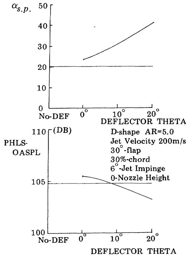
Figure 22 The effect of deflector angle variation on PHLs-OASPL and the parameter  $\alpha_{s.p.}$
