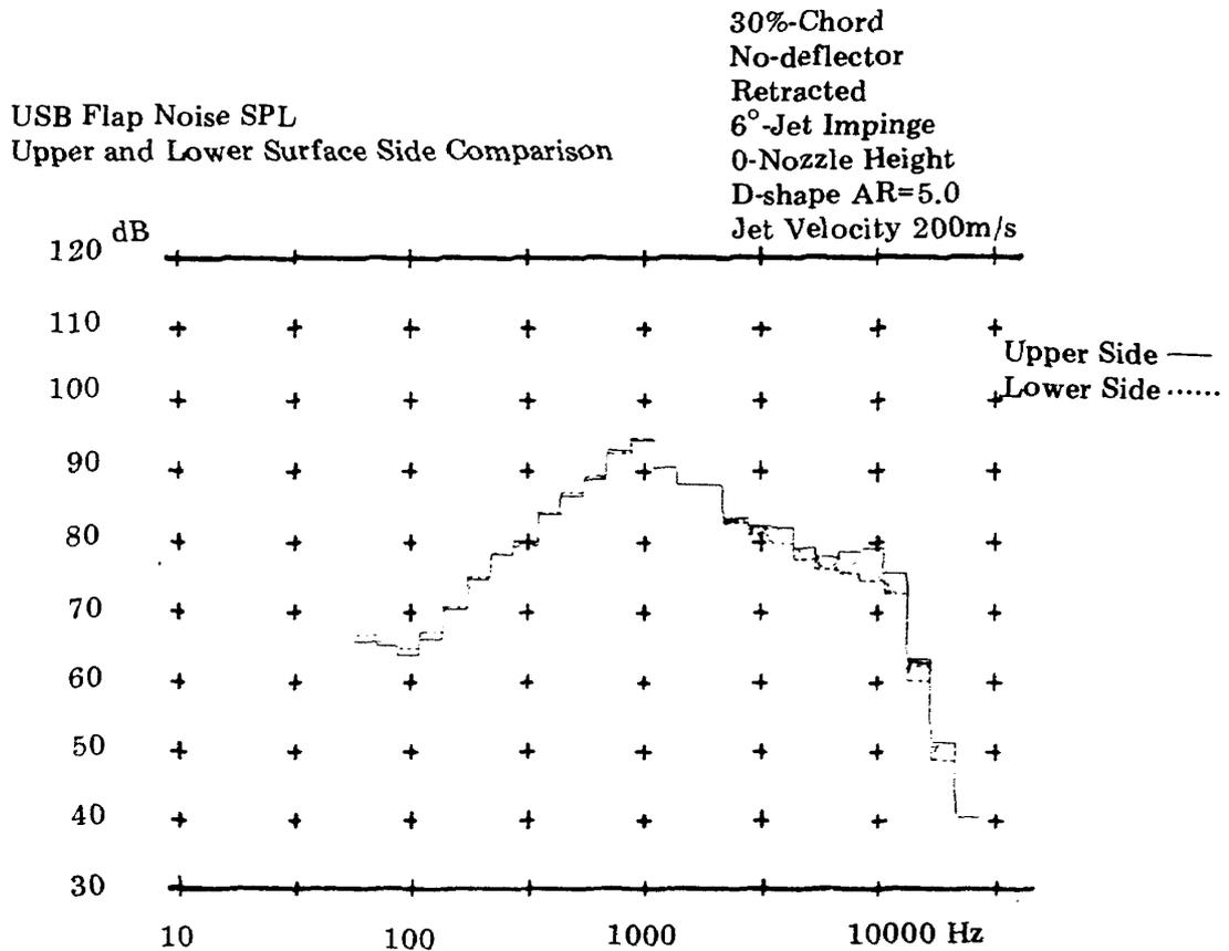
Figure 14 Comparison of 1/3 Octave-band spectra of USB-PHLS noise in the directions perpendicular to flap trailing edge
