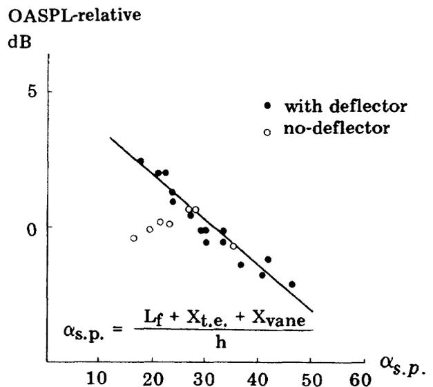
JET FLOW SPREADING PARAMETER DEFINED AS:
