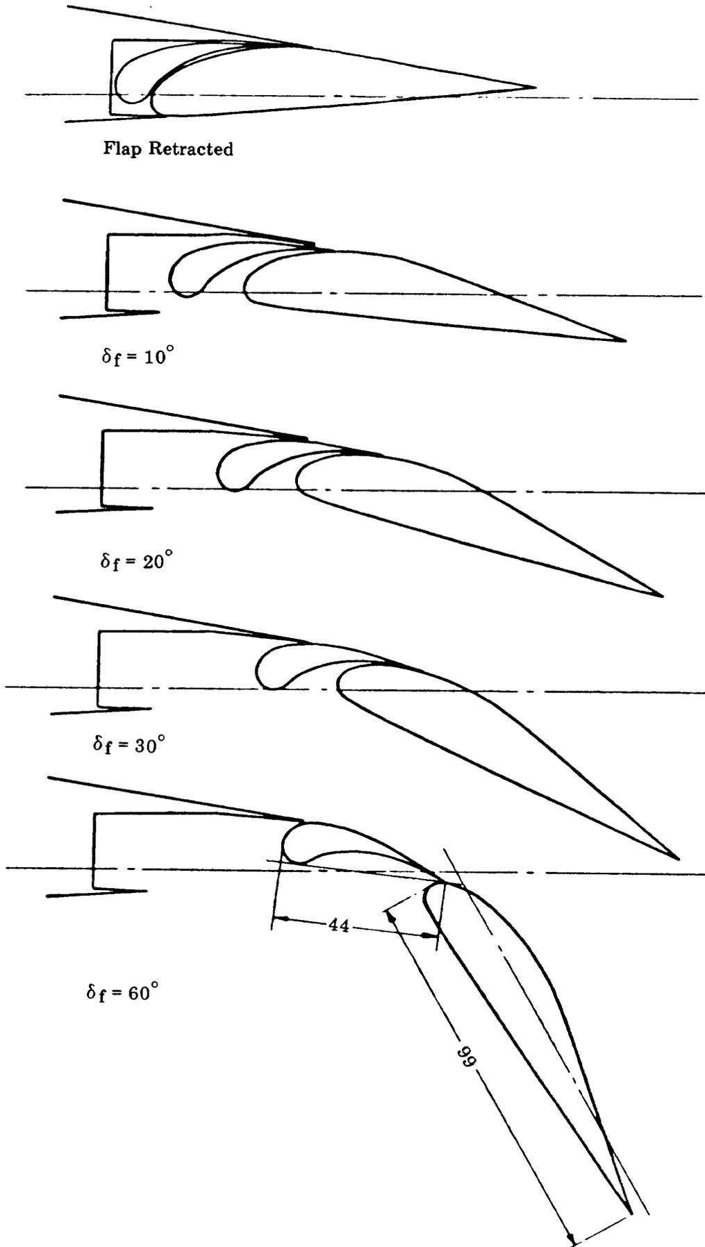
Figure 5 USB flap configurations
