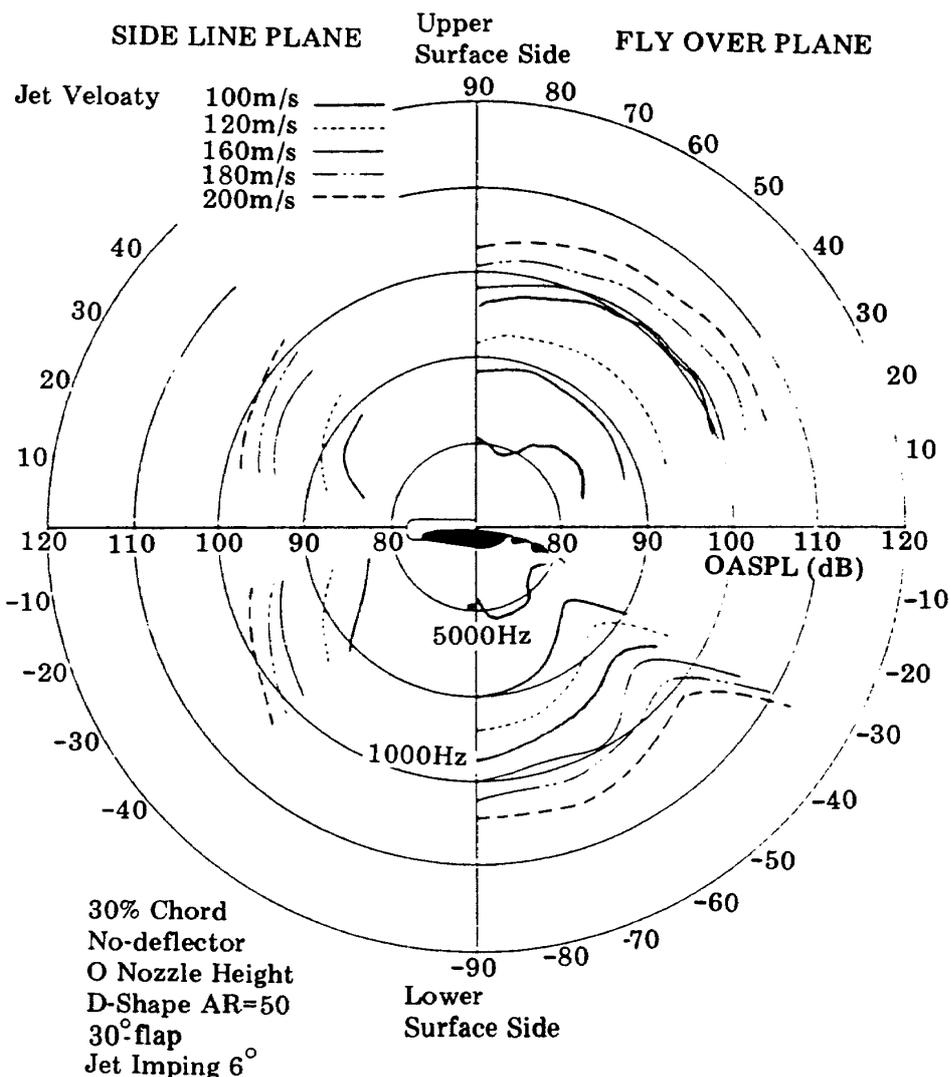
Figure 10 USR-PHLS noise directivity patterns and the effect of exhaust jet velocity variations
