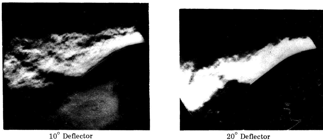
Figure 18-3 Flow visualization photographs by Schlieren (effect of deflector)
