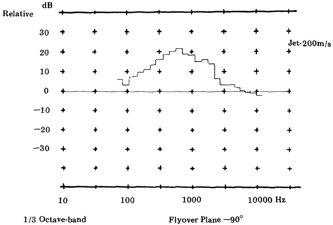
Figure 13 USB-PHLS relative noise SPL spectra as jet alone noise being baseline
