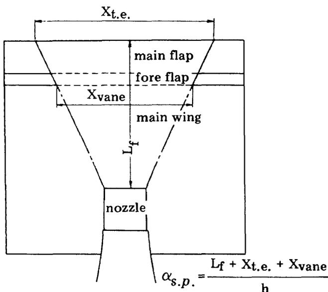
JET FLOW SPREADING PARAMETER
