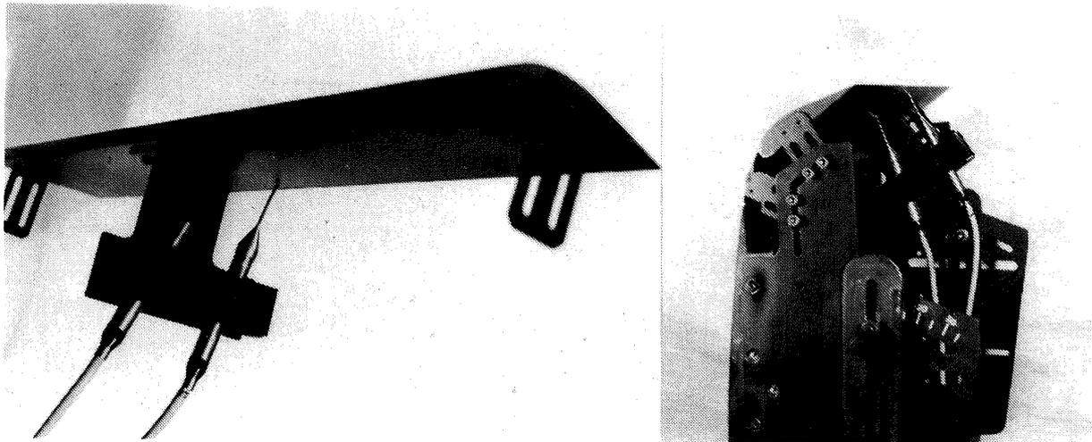
Photograph 2 Probe microphones installed at the main flap
