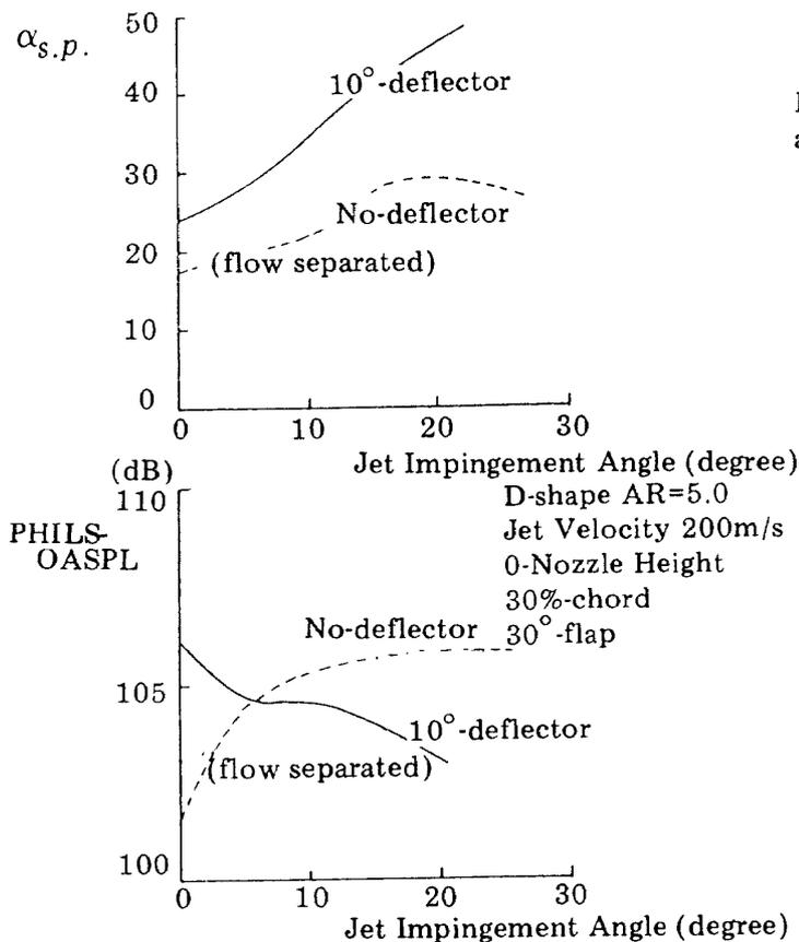
Figure 23 The effect of jet impingement angle variation on PHILS-OASPL and  $\alpha_{s.p.}$
