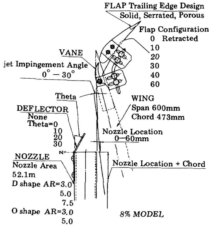
Figure 3 Parameters defining USB-PHLD system configurations
