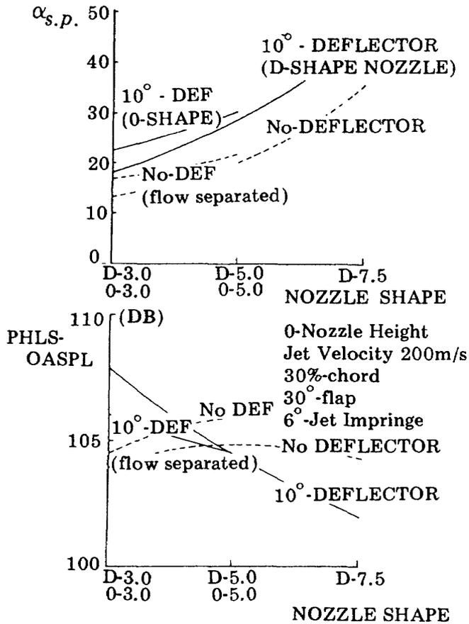
Figure 21 The effect of nozzle exit shape on PHLs-OASPL and the parameter  $\alpha_{s.p.}$
