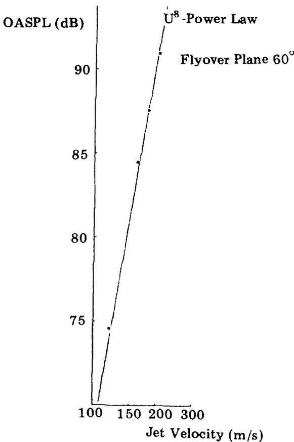
Figure 11 Overall Sound Pressure Level of jet alone case dependence on jet velocity
