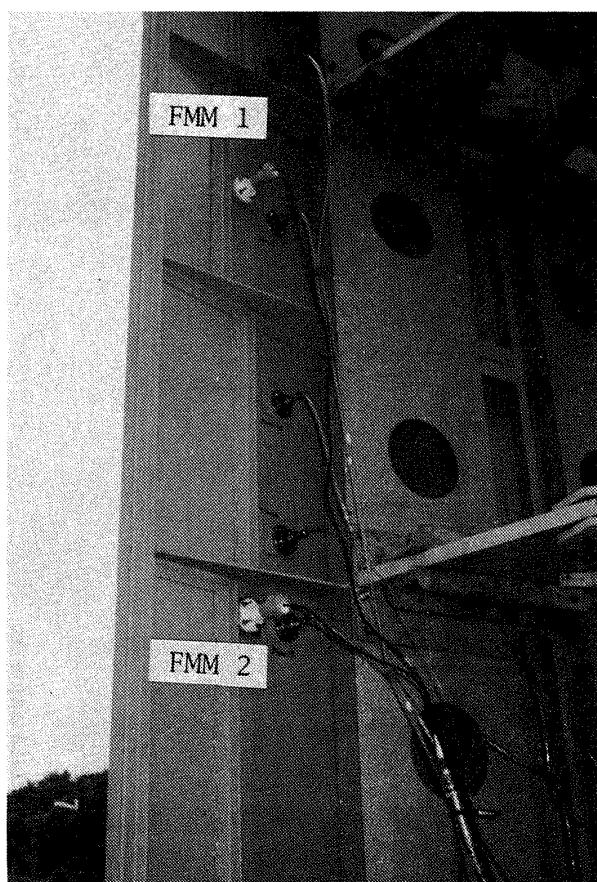
Photograph 4 Flush mounted microphones with teflon-coated adaptor
