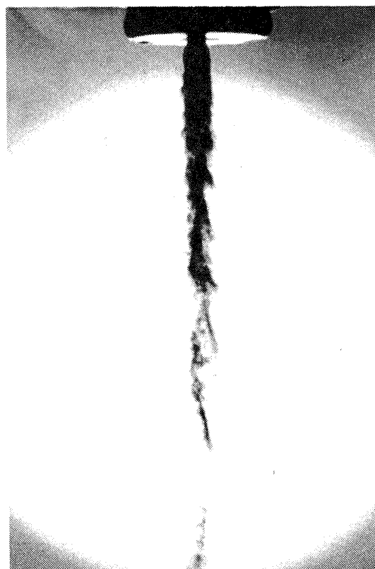
図 9.3 液体窒素 / ガス窒素 \left( \begin{array}{ll} u_{g0} = 256 \text{ m/s} & w_{g0} = 4.87 \text{ g/s} \\ u_{l0} = 15.18 \text{ m/s} & w_{l0} = 46.4 \text{ g/s} \end{array} \right)
