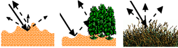
(a) Single-bounce (b) Double-bounce (c) Volume Fig.1. Typical Scattering Mechanism
