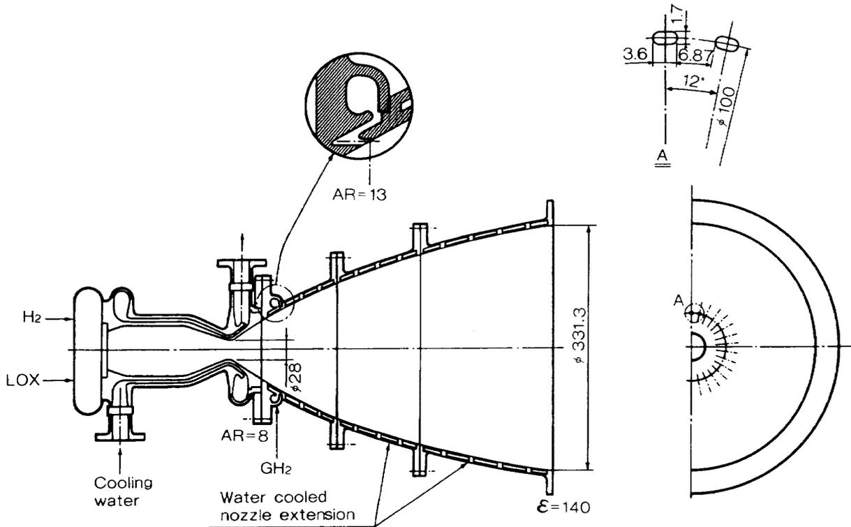
Fig. 1 Thrust chamber assembly
