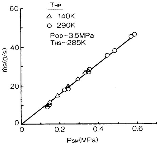
Fig. 3 Secondary flow rate vs. manifold pressure
