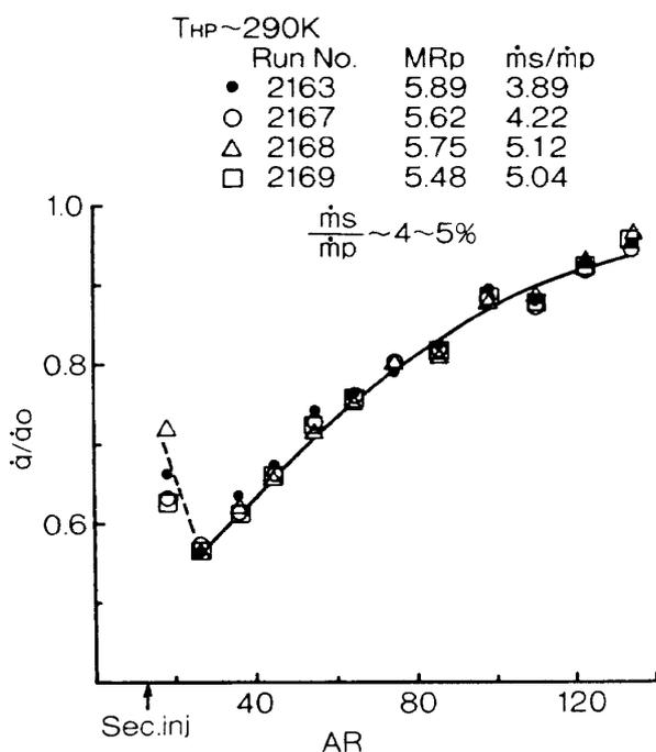
Fig. 7 Heat flux ratio for 4 to 5% secondary mass flow ratio
