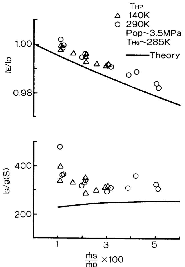
Fig. 6 Effective secondary flow specific impulse
