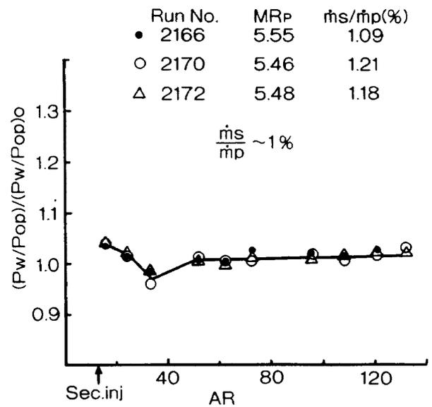
Fig. 4 Nozzle wall static pressure ratio for a secondary flow ratio of 1%
