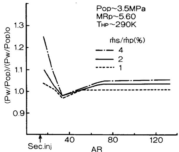
Fig. 5 Effect of secondary flow ratio on nozzle wall static pressure ratio
