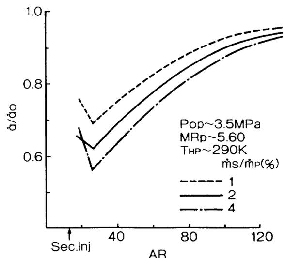
Fig. 8 Effect of secondary flow ratio on heat flux ratio
