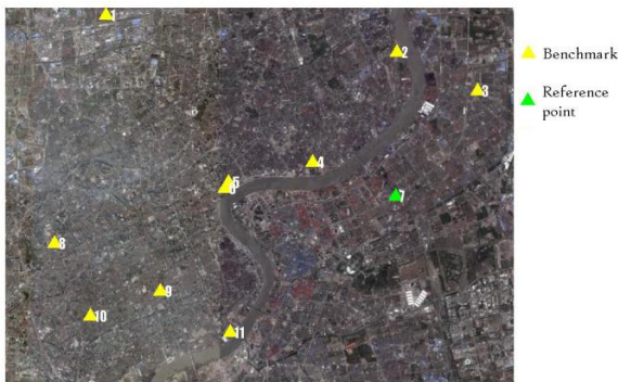
Fig. 4 Test area in Google earth and distribution of leveling benchmarks (the triangles). The green one is chosen as reference point for interferometry.
