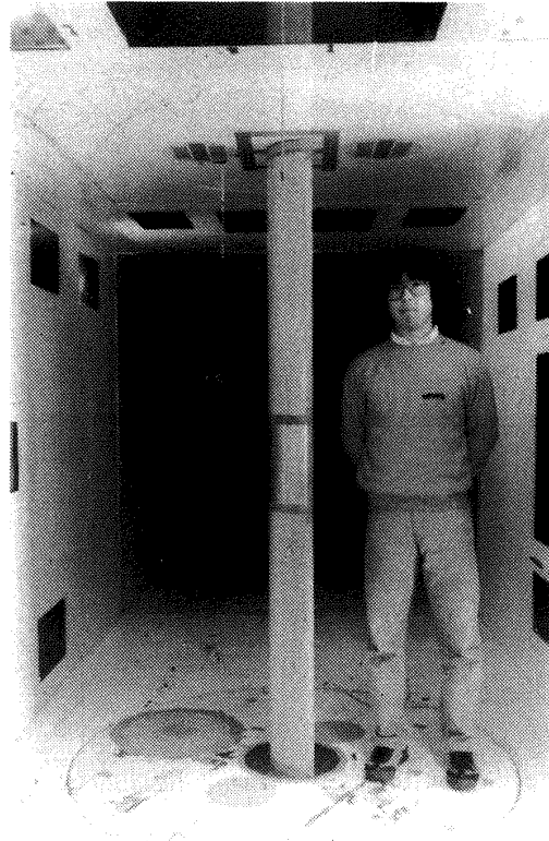
(b) Long large model in NAL Gust Wind Tunnel (front view) 航技研突風風洞中の長大模型(前方)
