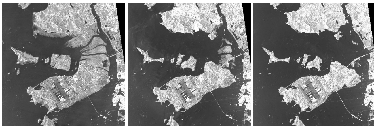
Figure 8. TerraSAR-X images acquired on 17 April 2009 (left), 28 April 2009 (center), and 14 November 2008 (right). Tide levels were 466 cm, 756cm, and 806 cm, respectively.
