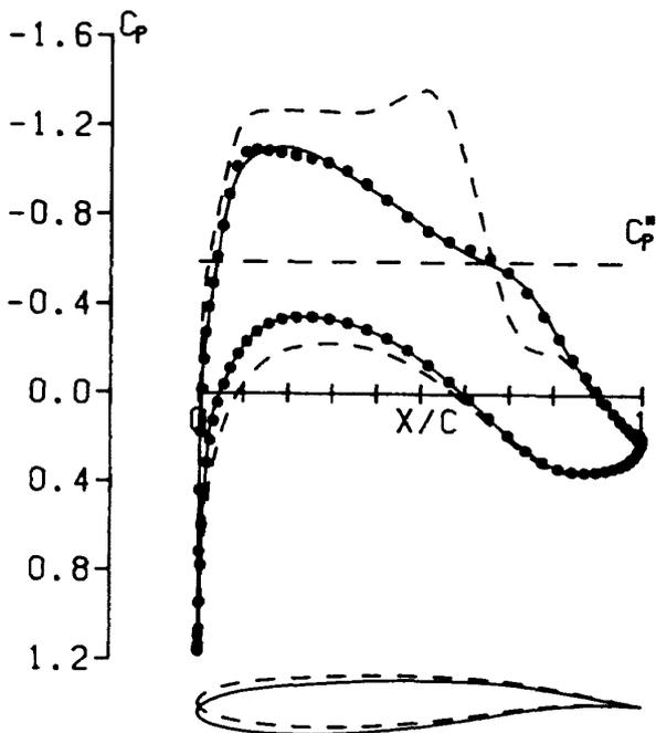
Fig. 3 Comparison of pressure distributions and geometries between designed (solid line), basic (dashed line) and target (dotted line), Case I.
