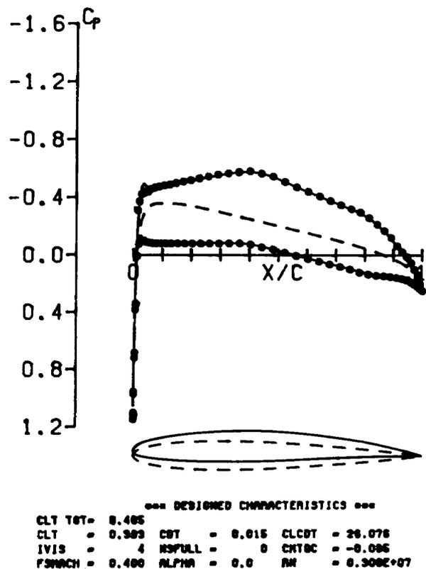
Fig. 12 Pressure distribution of designed airfoil at mode 3, Case IV.
