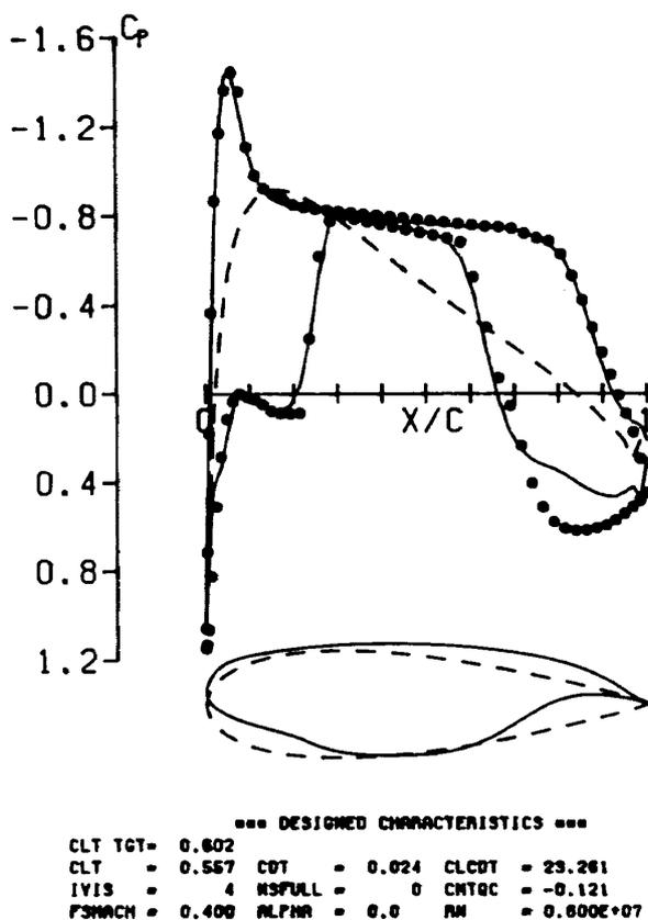
Fig. 13 Pressure distribution of designed airfoil with trailing edge modification at mode 3A, Case V.
