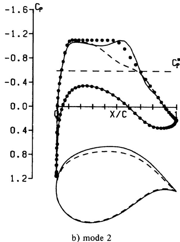
Fig. 7 Iterative history of design and pressure recovery, Case II.
