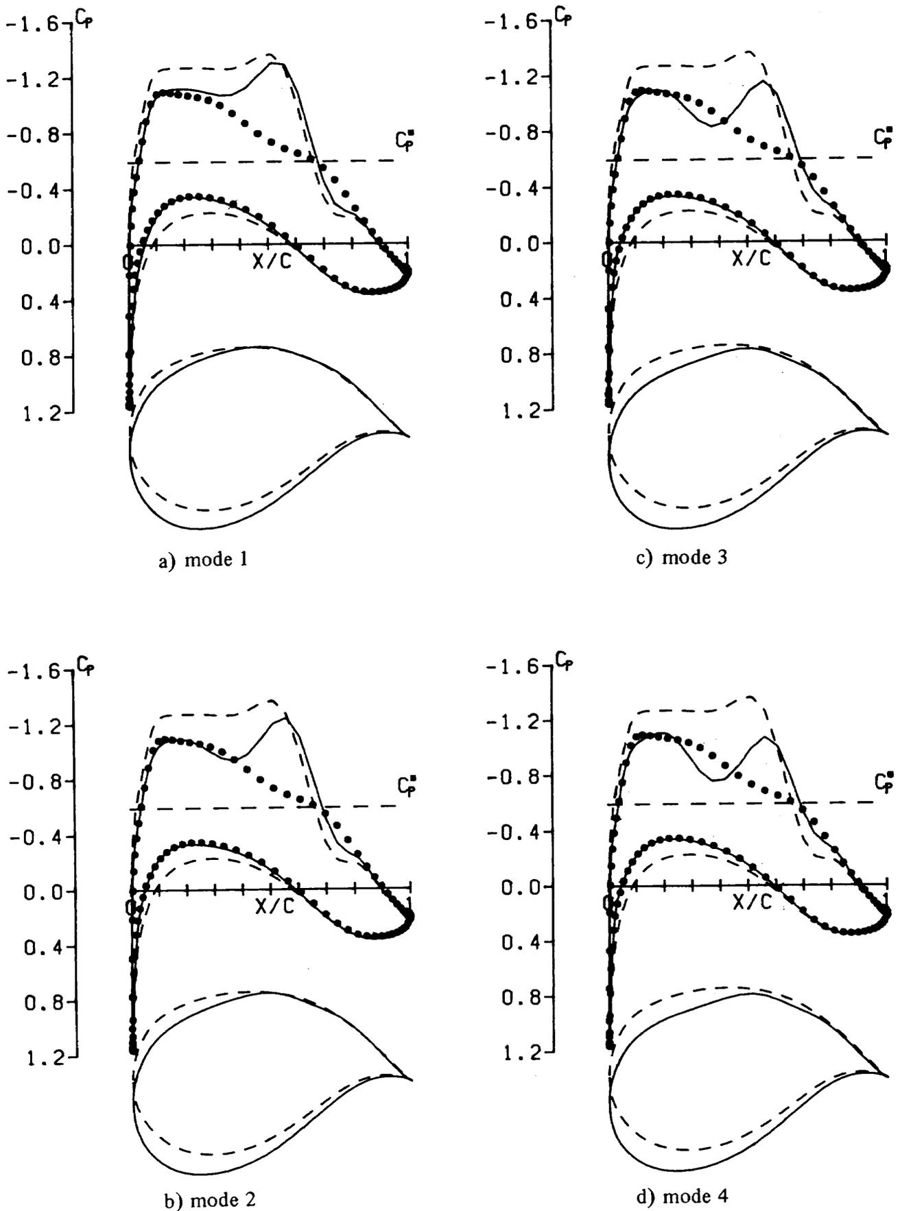
Fig. 5 Iterative history of design and pressure recovery, Case I.
