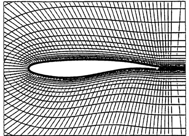
Fig. 1. Computational grid generated about transonic airfoil.
