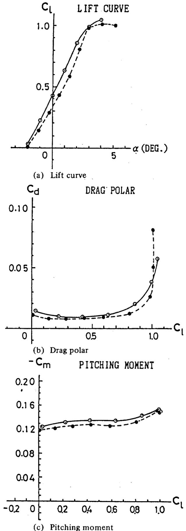
Fig. 5. Aerodynamic force comparison ( $Re = 23 \times 10^6$ ,  $M = 0.75$ ). Open circles for NSFOIL computation and filled circles for experiments.
