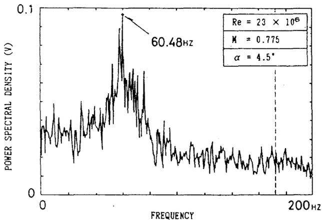
Fig. 13. Experimental result of oscillatory motion – power spectrum density ( $Re = 23 \times 10^6$ ,  $M = 0.775$ ,  $\alpha = 4.5^\circ$ ).
