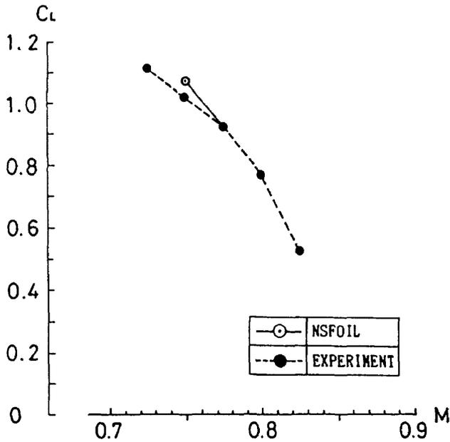
Fig. 11. Buffet boundary comparison ( $Re = 23 \times 10^6$ ).
