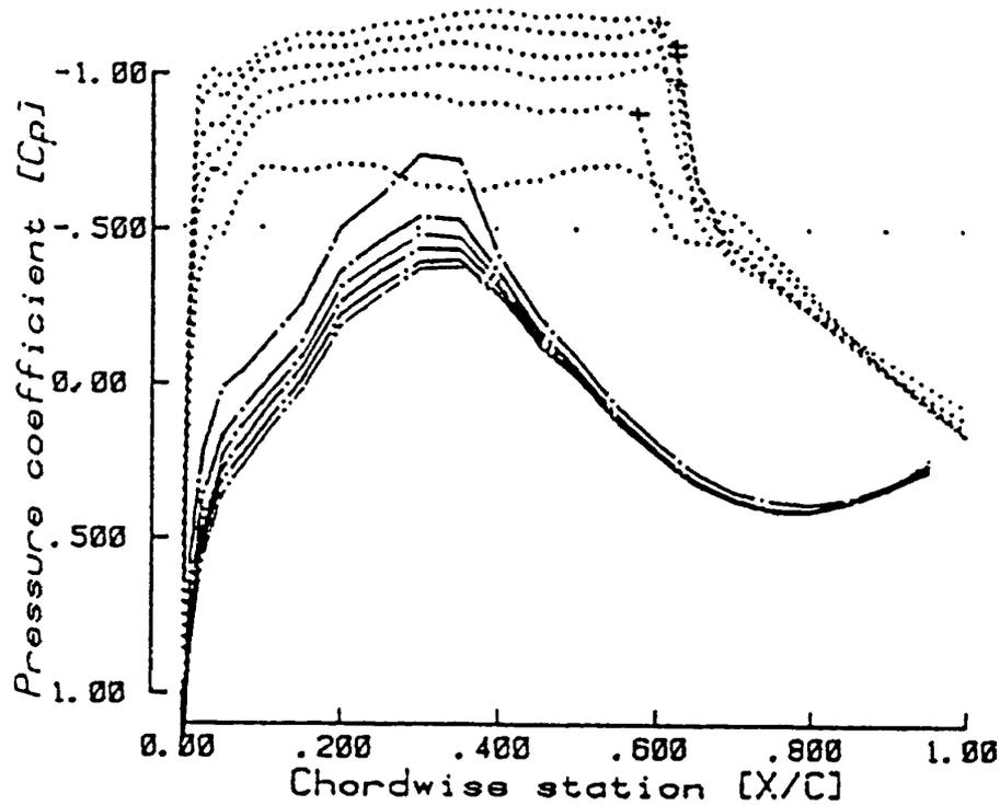
(a) Pressure distribution. Dotted line for upper surface and solid line for lower surface.
