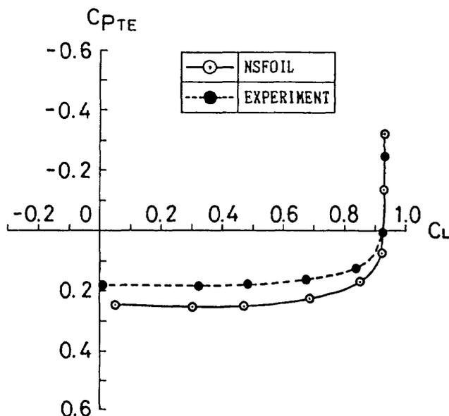
Fig. 10. Trailing edge pressure comparison ( $Re = 23 \times 10^6$ ,  $M = 0.775$ ).
