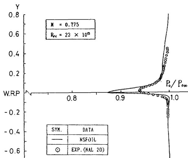
Fig. 9. Wake profile comparison ( $Re = 23 \times 10^6$ ,  $M = 0.775$ ,  $\alpha = 3.0^\circ$ ).
