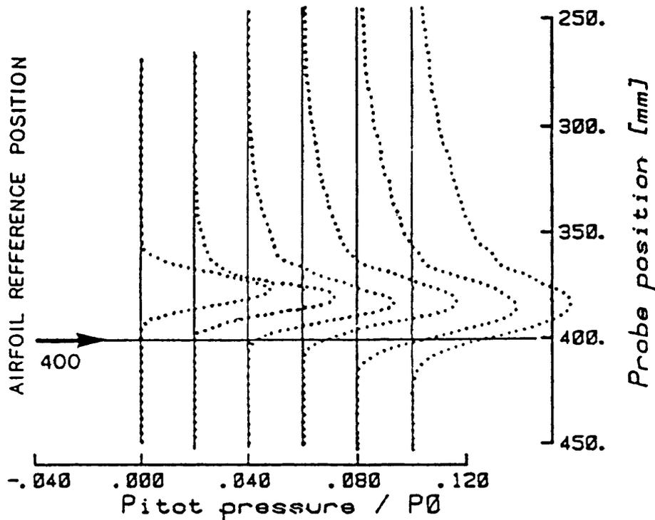
(b) Wake profile. Dotted line for wake profile and solid line for reference.
