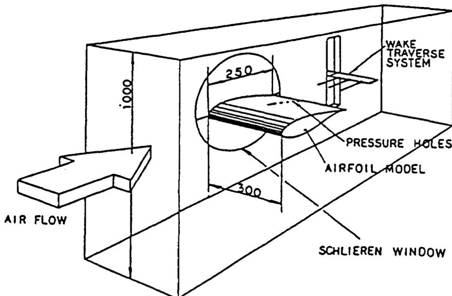
Fig. 3. Schematics of wind tunnel test.
