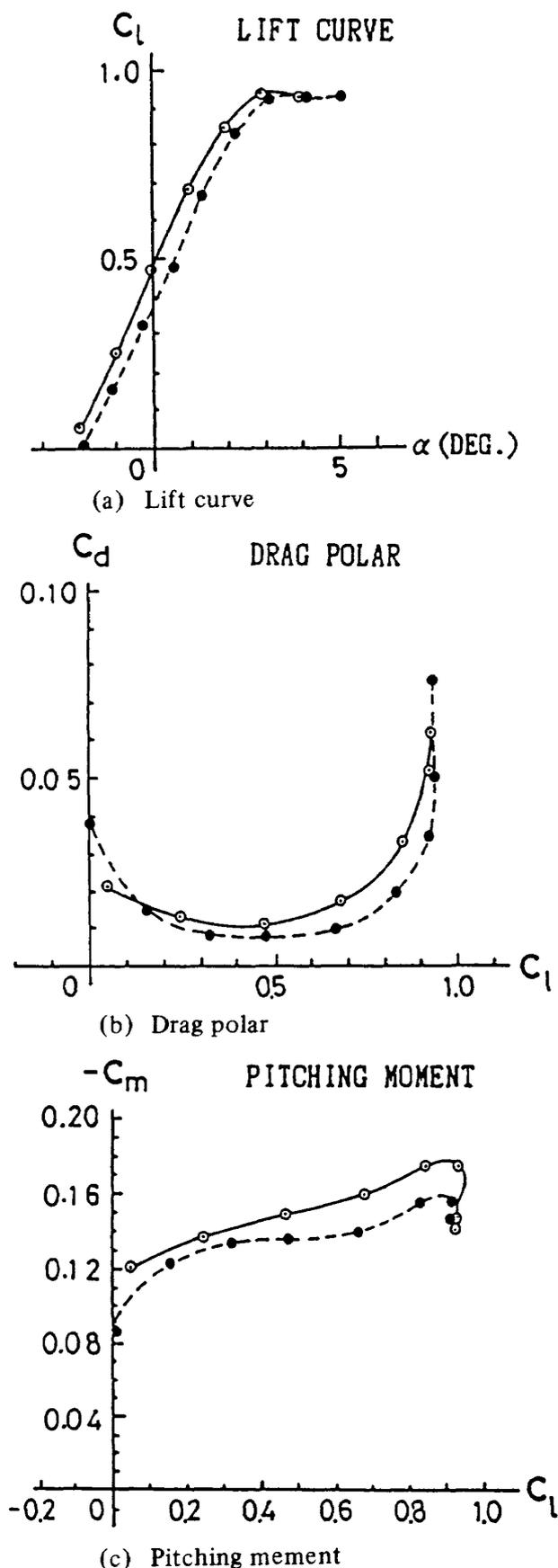
Fig. 6. Aerodynamic force comparison ( $Re = 23 \times 10^6$ ,  $M = 0.775$ ).
