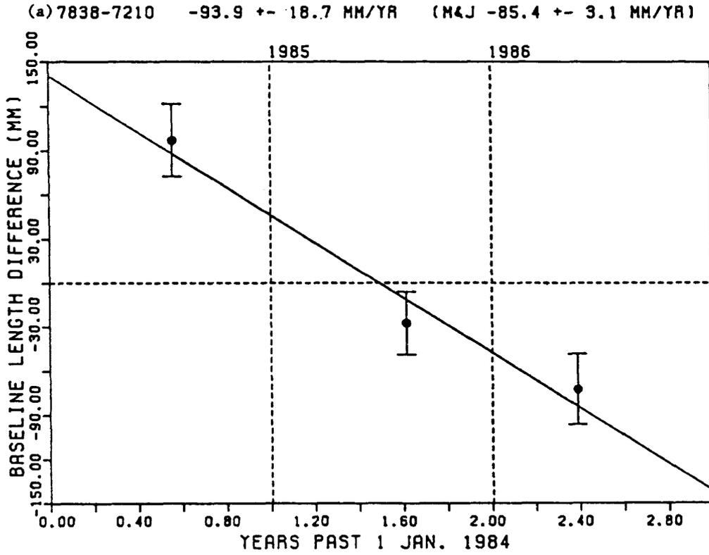
Fig. 10a Baseline Length Differences from the Nominal Value between Shimosato and Haleakala
