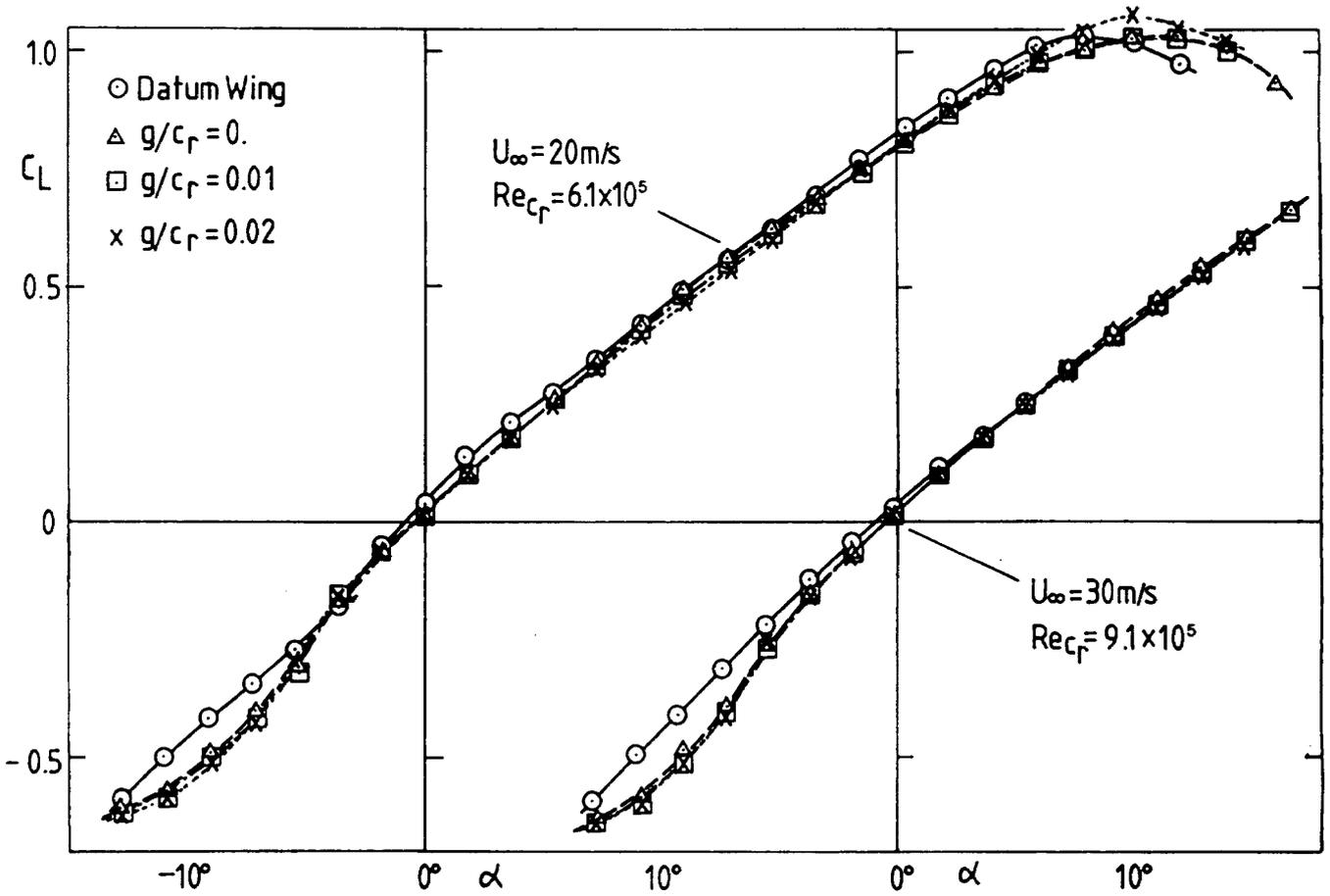
Fig. 12 Effect of Vortex Plate on  $C_L$  vs.  $\alpha$
