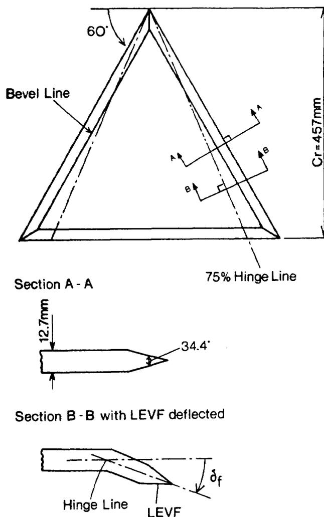
Fig. 2 Delta Wing Model with LEVF
