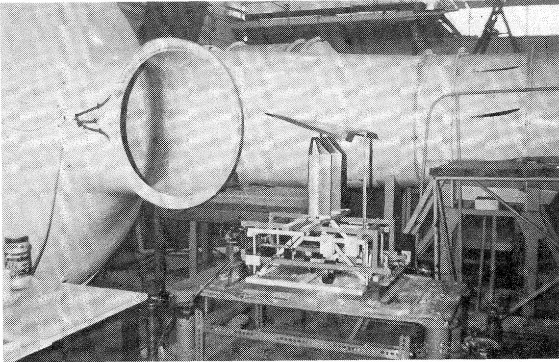
Fig. 4 Wind Tunnel, Model Mounting and Tunnel Balance
