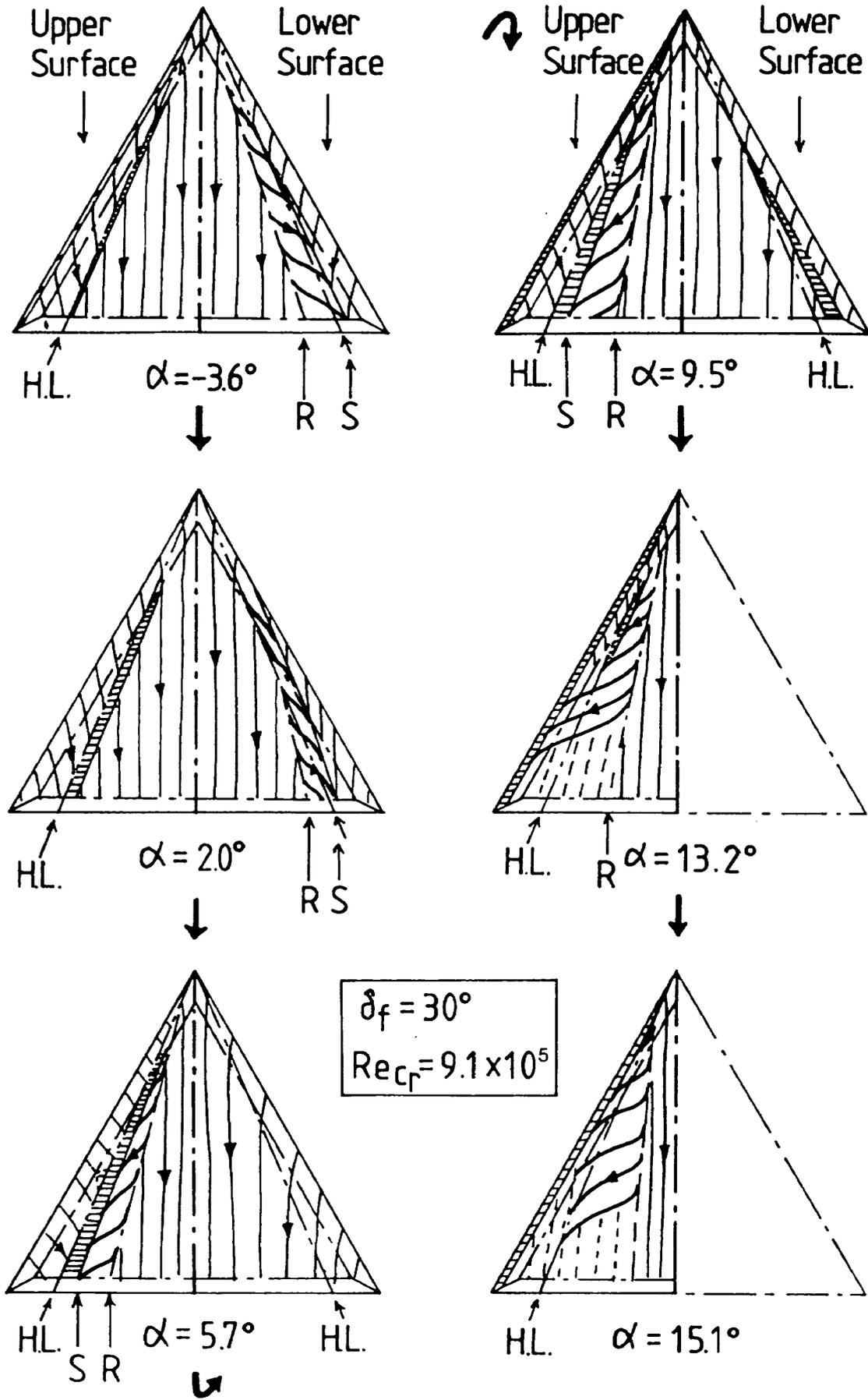
Fig. 9 Surface Flow Patterns ( $\delta_f = 30^\circ$ )
