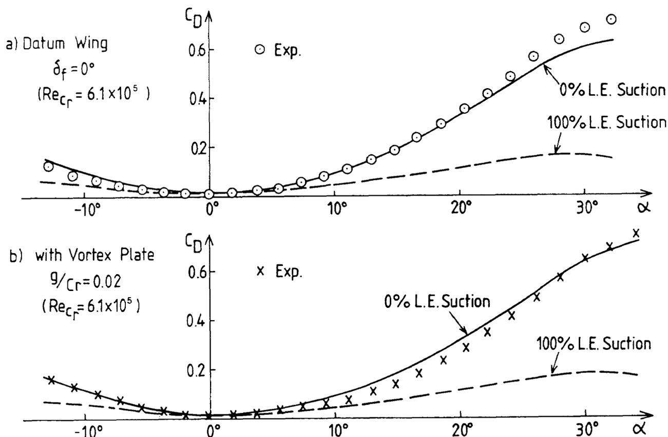
Fig. 16 Effect of Leading-Edge Suction Force on  $C_D$  (Datum Wing &  $g/C_r = 0.02$ )
