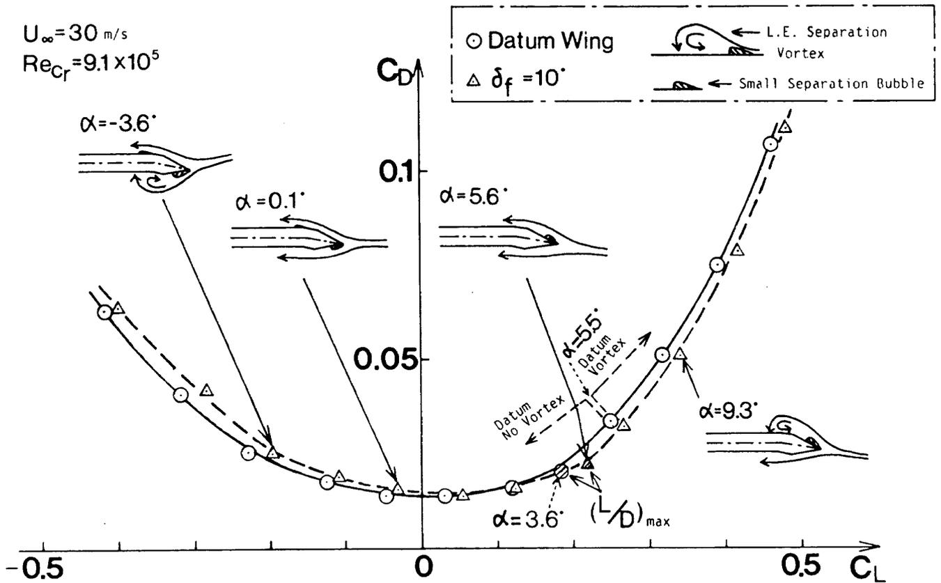
Fig. 10  $C_D$  vs.  $C_L$  and Cross Flow Patterns ( $\delta_f = 10^\circ$ )
