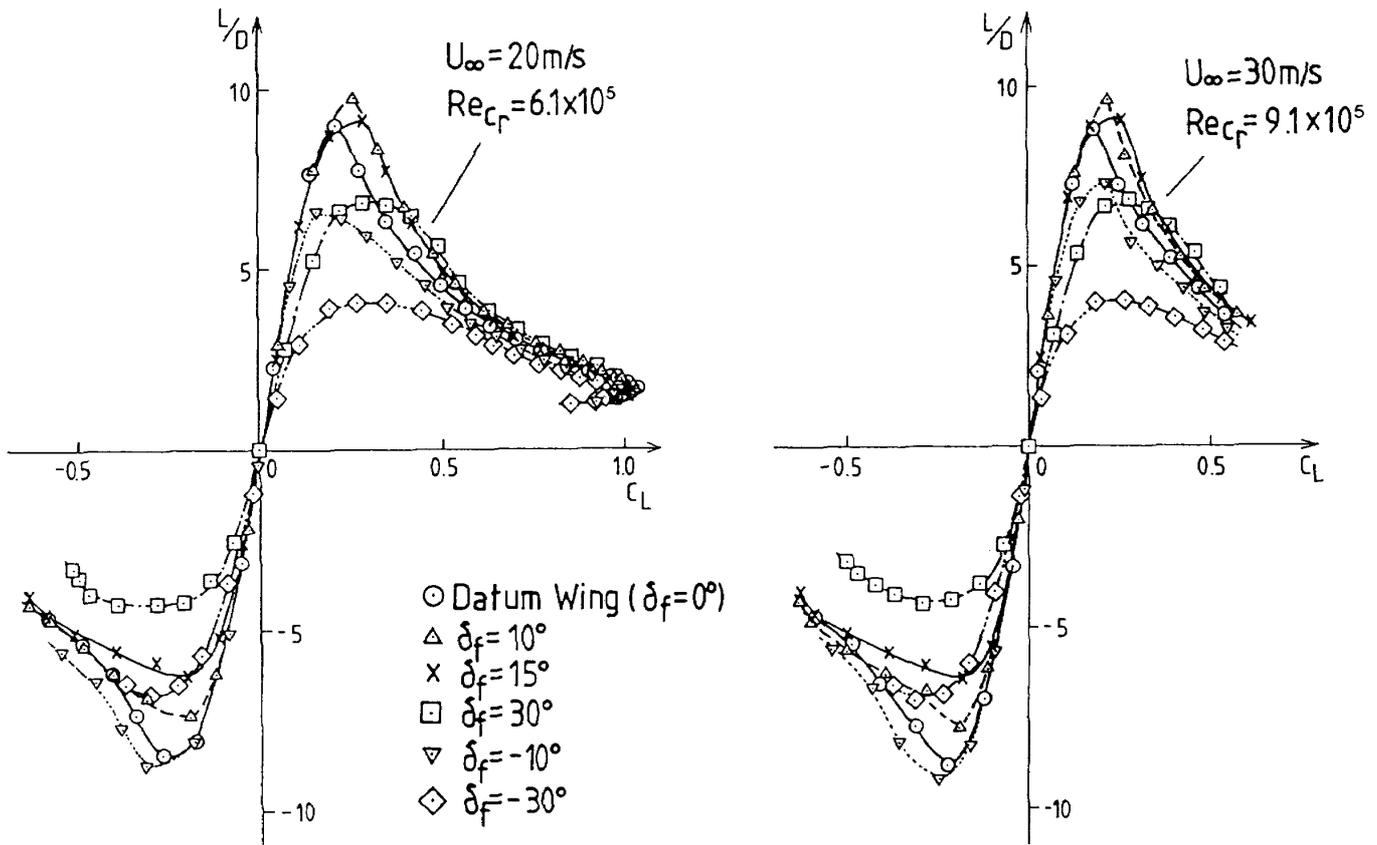
Fig. 7 Effect of LEVF on  $L/D$  vs.  $C_L$
