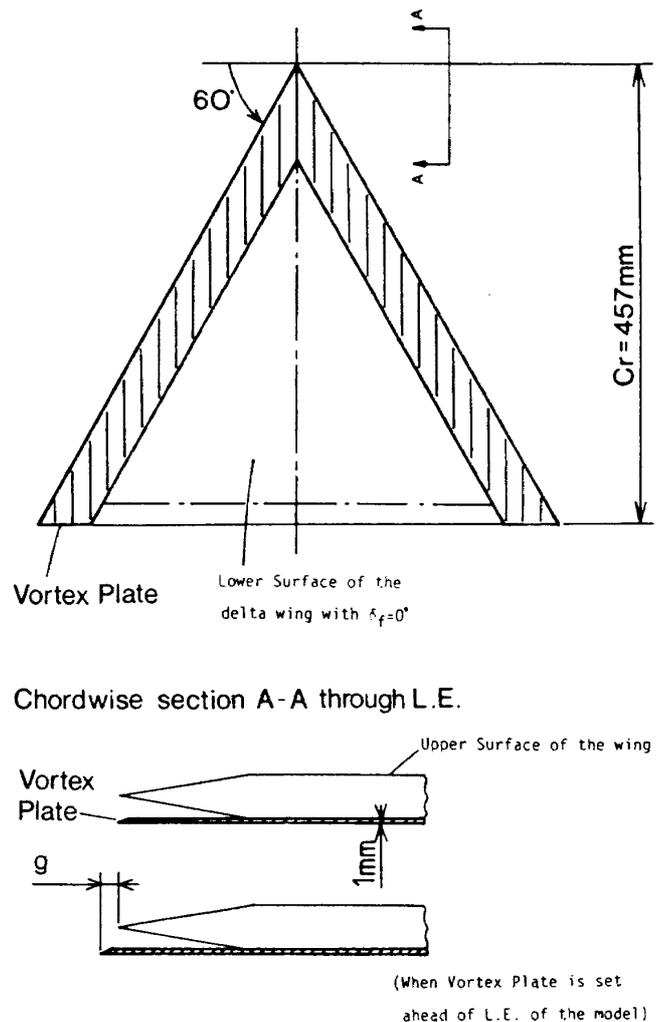
Fig. 3 Delta Wing Model with Vortex Plate
