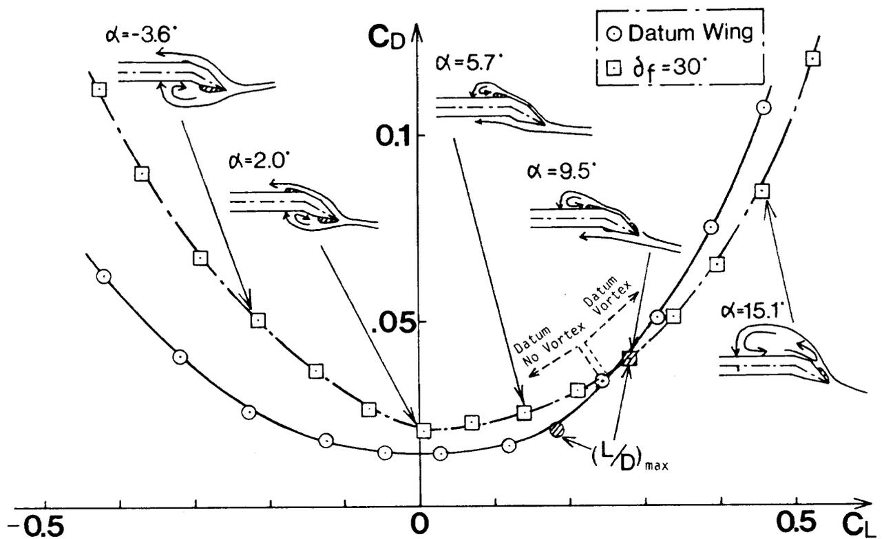
Fig. 11  $C_D$  vs.  $C_L$  and Cross Flow Patterns ( $\delta_f = 30^\circ$ )
