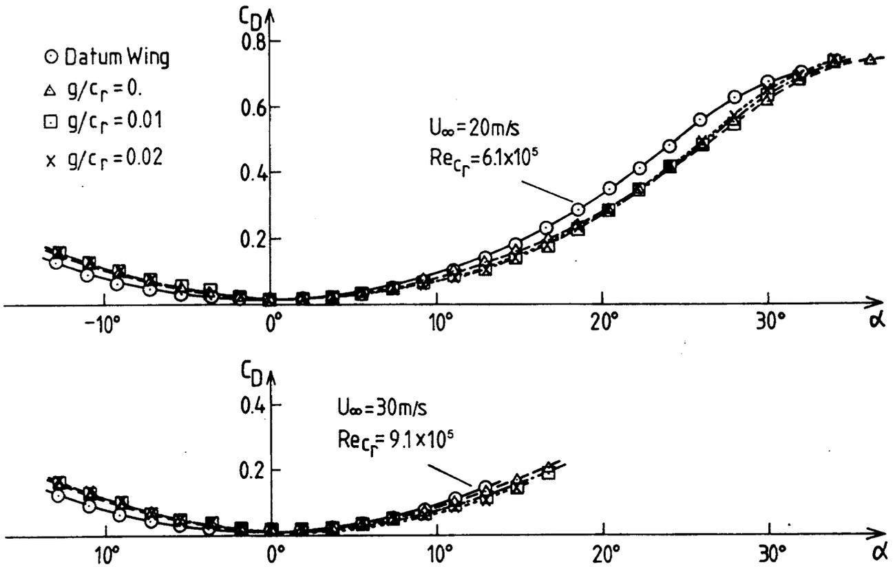
Fig. 13 Effect of Vortex Plate on  $C_D$  vs.  $\alpha$
