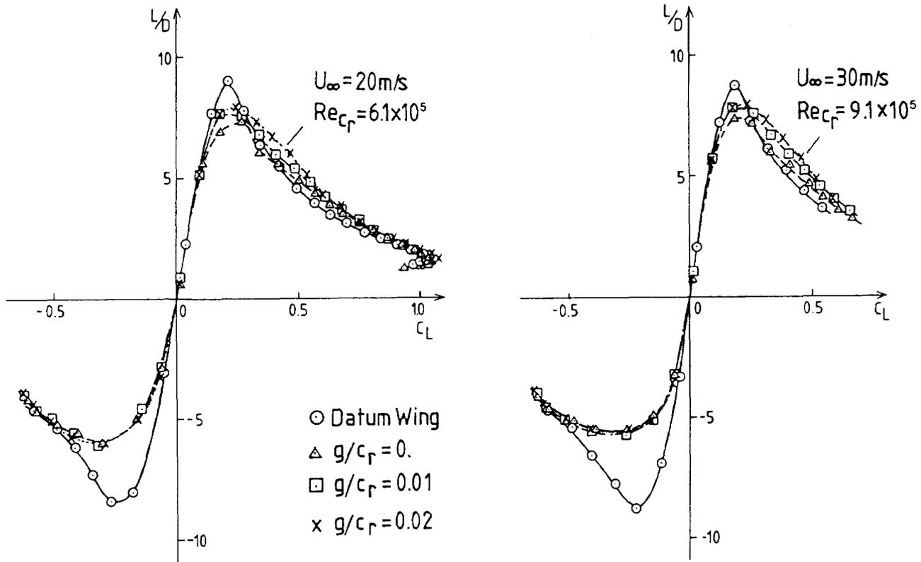
Fig. 14 Effect of Vortex Plate on  $L/D$  vs.  $C_L$
