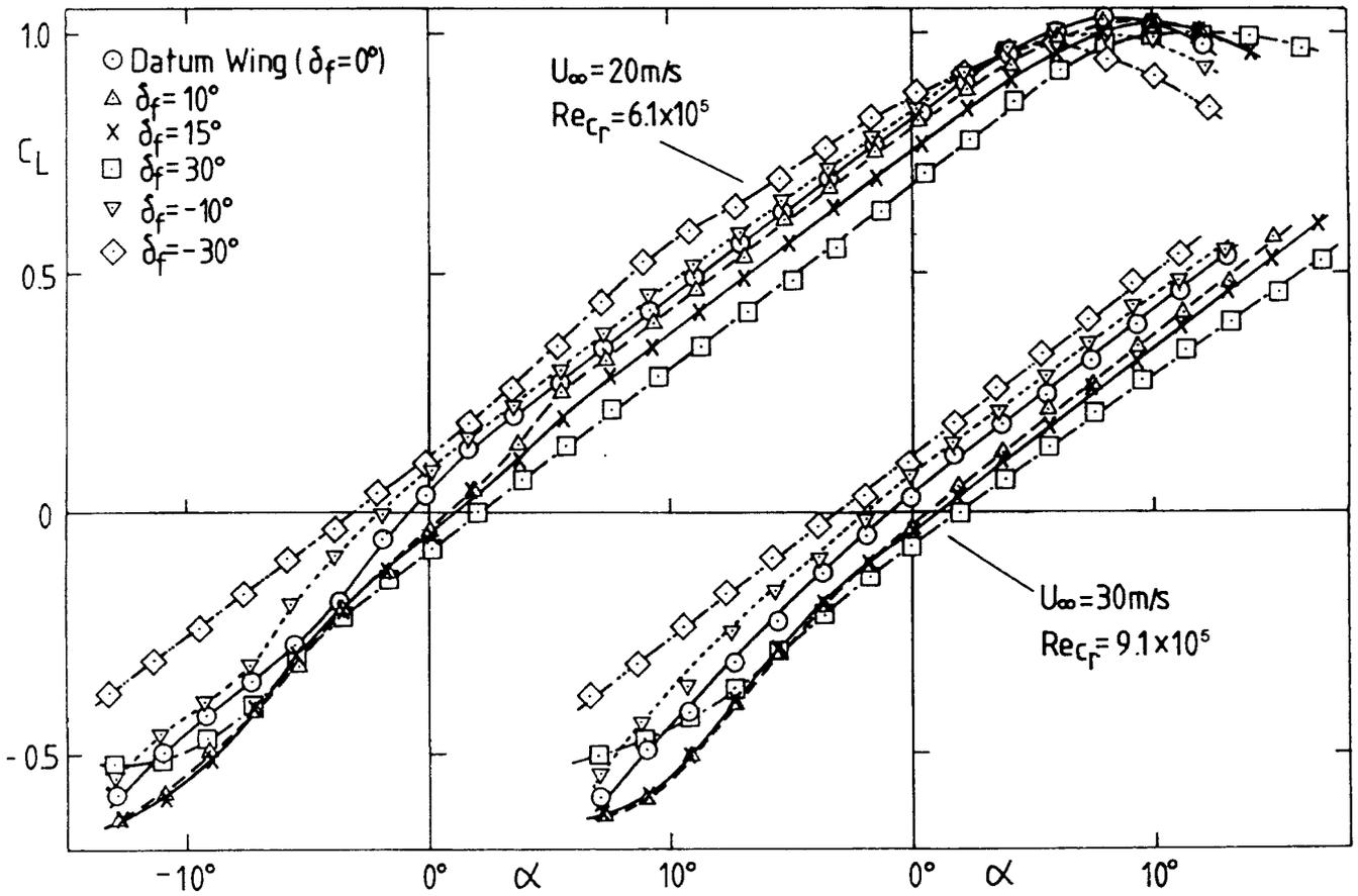
Fig. 5 Effect of LEVF on  $C_L$  vs.  $\alpha$
