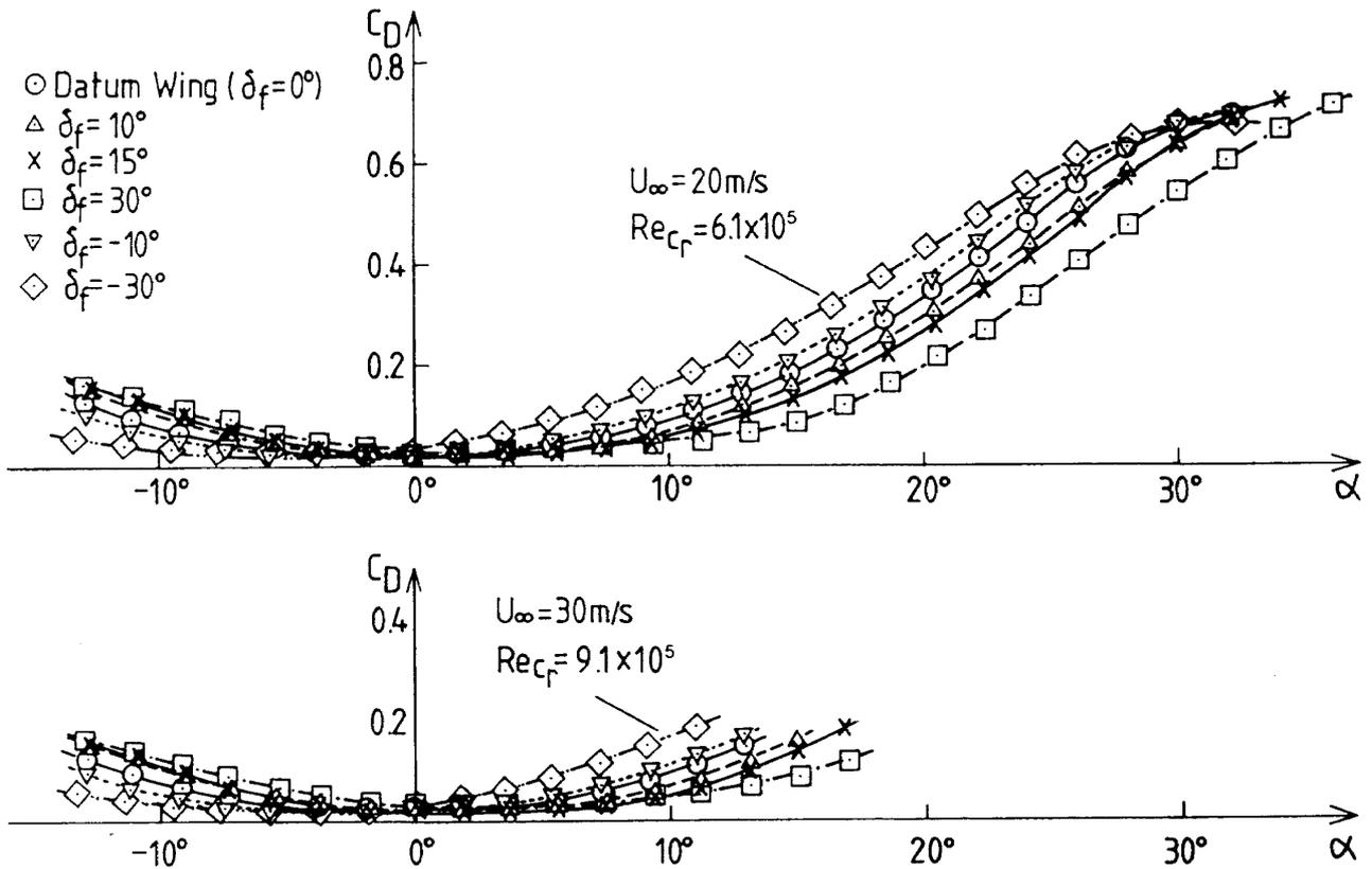
Fig. 6 Effect of LEVF on  $C_D$  vs.  $\alpha$
