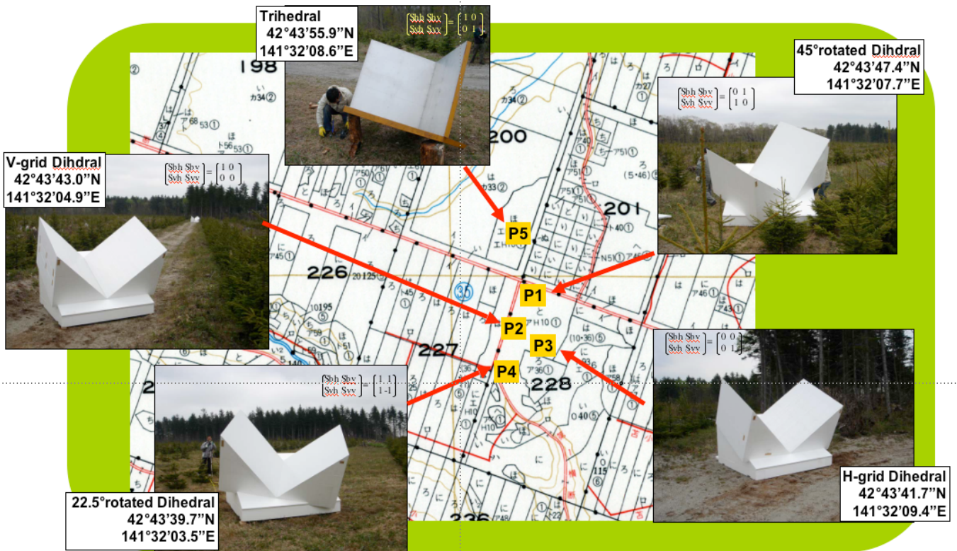
Fig. 2 Location of calibration targets in the Tomakomai forested field.
