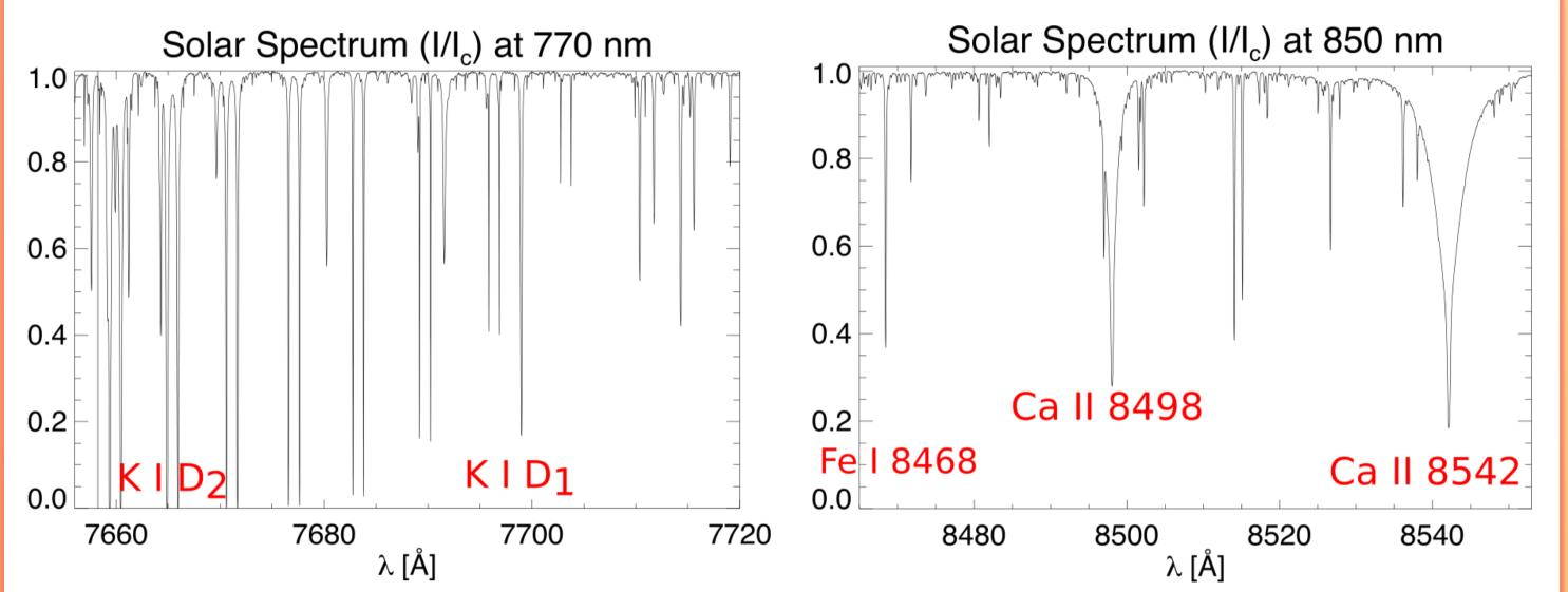
These spectral windows contain two of the most capable lines to understand the <u>dynamics</u> of the upper photosphere (K I  $D_1$ ) and the <u>magnetism</u> of the solar chromosphere (Ca II 8542 Å). In addition, thanks to the balloon conditions, we can have access for the first time to K I  $D_2$ , a spectral line blocked by telluric  $O_2$  absorption.
