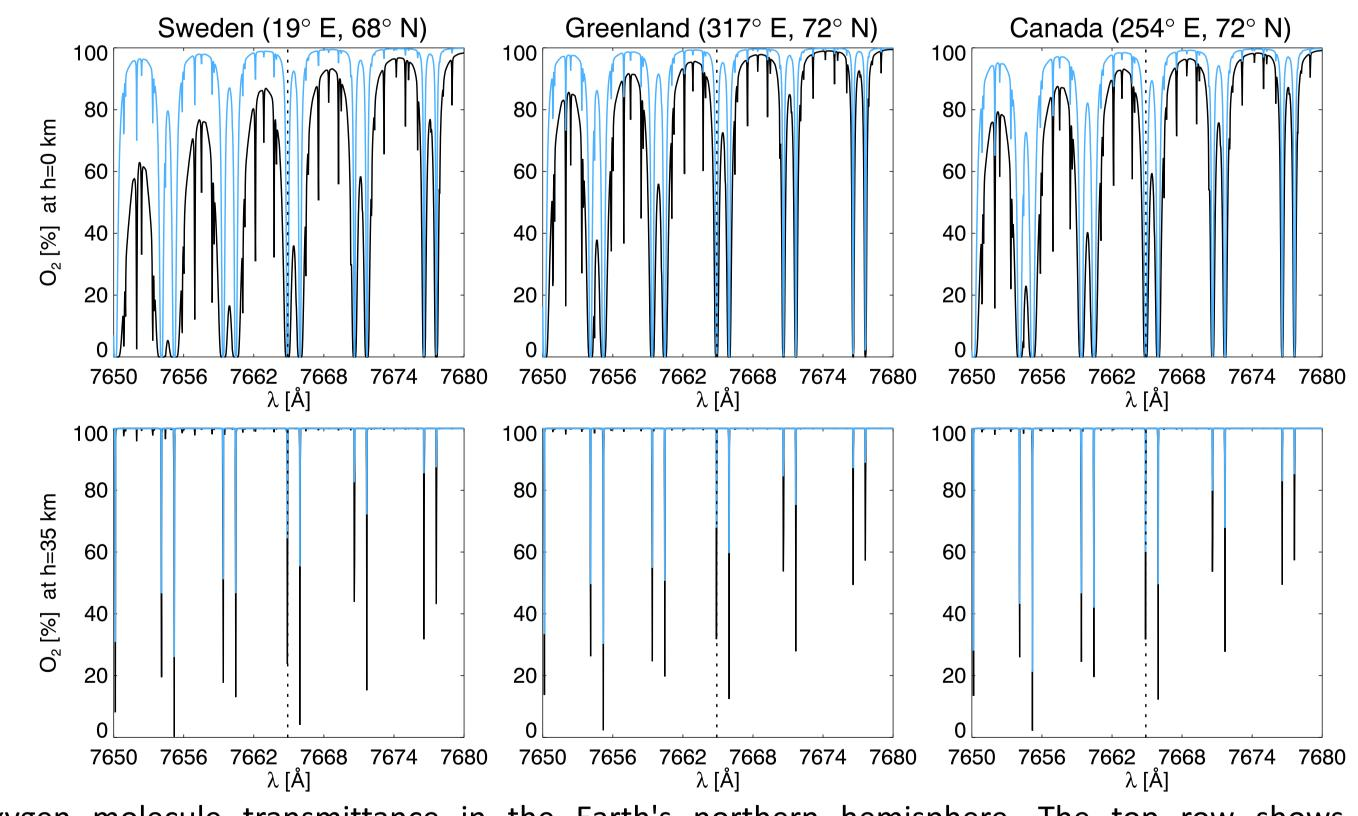
Oxygen molecule transmittance in the Earth's northern hemisphere. The top row shows the transmittance at ground level while the bottom row corresponds to the results for an observatory at 35 km above the sea level. Blue designates daytime while black corresponds to a reference night time.
