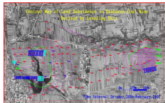
Fig.2 Distribution of bench marks in Dashucun coal mine and one contour map of land subsidence derived by the leveling data
