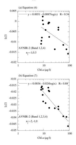
Figure 4 Relationship between LCI from AVNIR-2 using Equation (6), (7) and in-situ Chl-a.
