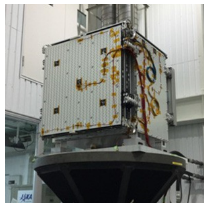
Vibration Test of SAR Antenna and Satellite Body
