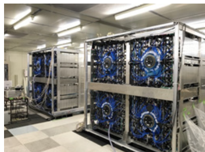
Prototype of SSPA (consisting of a pair of power amplifiers)
