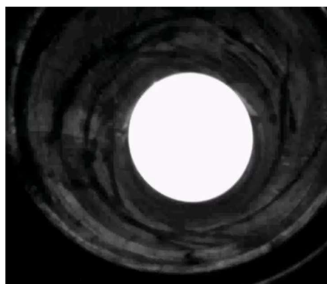
Fig. 5. Molten Pt droplet levitated by Gas-jet method
