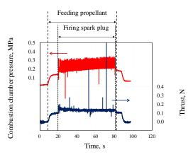
Fig. 6. Time history of combustion experiment: intermittent combustion
