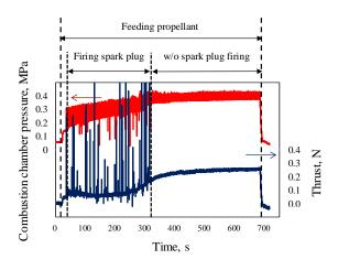
Fig. 7. Time history of firing spark plug with stable combustion
