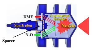
Fig. 1. Schematic of the prototype thruster
