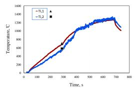
Fig. 10. Time histories of estimated temperature on the inner wall
