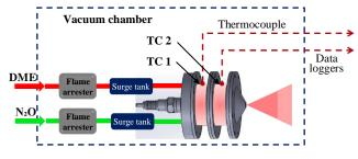
Fig. 5. Schematic of the detailed information of the experiment apparatus
