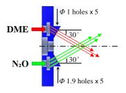
Fig. 2. Schematic of the impingement-type  $N_2O/DME$  injector.
