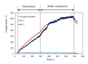
Fig. 8. Time histories of the outer surface temperature of the thrust chamber
